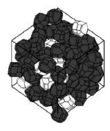
**Fig. 24** example of stochastically simulated LiFePO<sub>4</sub> agglomerate morphology. Reprinted with permission from ref. 217. Copyright 2011, The Electrochemical Society.
