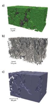
Fig. 29 3D reconstructions obtained by FIB tomography of (a) a LiFePO<sub>4</sub> composite positive electrode, (b) a glass fiber separator and (c) a graphite negative electrode. Reprinted with permission from ref. 231. Copyright 2012, The Electrochemical Society.
