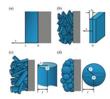
**Fig. 27** Song and Bazant's model electrode configurations, particle geometries, and corresponding coordinate systems, where the blue region and the gray region represent the active material and the current collector, respectively: (a) thin film electrode, (b) electrode with planar particles, (c) electrode with cylindrical particles, and (d) electrode with sphere particles. Reprinted with permission from ref. 223. Copyright 2013, The Electrochemical Society.
