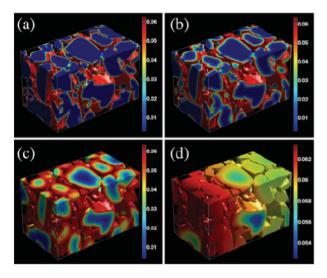
Fig. 30 Li concentration (mol cm<sup>-3</sup>) evolution during the discharge of a Li<sub>x</sub>CoO<sub>2</sub> microstructure at a constant voltage loading. Through electrochemical reaction, Li ions are injected into cathode particles: (a)–(d) corresponding to time of 4.04, 20.1, 133.3 and 1226.5 s (assuming the value of the diffusion coefficient of 10<sup>-10</sup> cm<sup>2</sup> s<sup>-1</sup>). Reprinted with permission from ref. 234. Copyright 2012, The Electrochemical Society.
