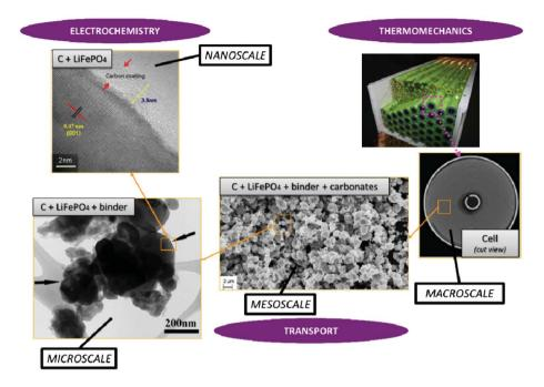
**Fig. 1** Schematics of the multiscale character of a LiFePO<sub>4</sub> electrode in a LIB and physicochemical mechanisms.<sup>24</sup> Schematics made with TEM and SEM pictures reported in ref. 25 (courtesy of X. Sun, University of Waterloo, Canada) and from the spiral battery tomography picture in ref. 26 (reprinted with permission of Elsevier).
