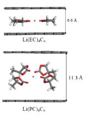
Fig. 22 the side views of optimized grapheme structures with intercalated solvated lithium, calculated by Tasaki et al. Reproduced with permission from ref. 215. Copyright 2012, The Electrochemical Society.
