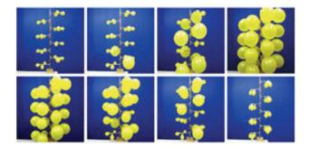
**Fig. 26** States of interconnected rubber balloons during loading and unloading with air *via* a pressure vessel. Reprinted from ref. 222 with permission of Elsevier.
