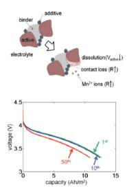
Fig. 21 top) Schematic diagram of the dissolution process: two Mn<sup>3+</sup> cations convert into one Mn<sup>4+</sup> and one Mn<sup>2+</sup>, then Mn<sup>2+</sup> ions leave the solid phase; down) calculated effect of dissolution and discharge voltage profiles for different numbers of cycles. Reprinted with permission from ref. 206. Copyright 2011, The Electrochemical Society.
