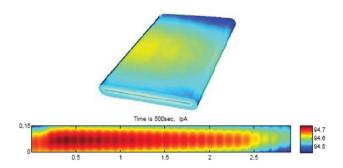
**Fig. 36** Reaction current density distribution after 500 s at 4C discharge of 20 Ah cell with continuous tabs at (a) surface and (b) unrolled jelly roll. Reproduced with permission from ref. 262. Copyright 2012, The Electrochemical Society.
