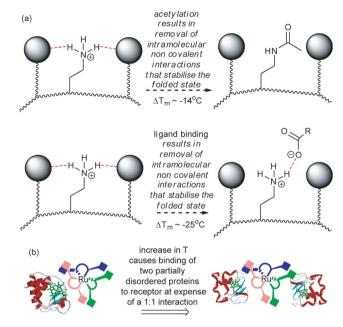
Fig. 4 Schematic depicting the basis of reduced  $T_{\rm m}$  in cyt c (a) post covalent modification and binding to surface receptors results in structural loosening in order to maximise non-covalent contacts (b) a change in stoichiometry results on increasing the temperature and is promoted by binding of more disordered proteins.
