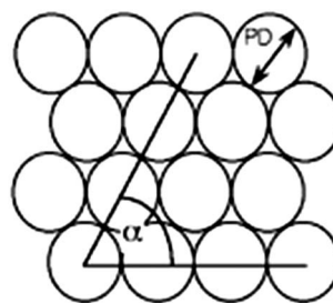
Fig. 8 The ideal hexagonal arrangement in the pores of a honeycomb structured porous film where alpha is the angle among three adjacent pores and PD is the pore diameter. Reprinted from S. D. Angus and T. P. Davis, Polymer surface design and infomatics: facile microscopy/image analysis techniques for self-organizing microporous polymer film characterization , Langmuir , 2002, 18 , 9547–9553.
