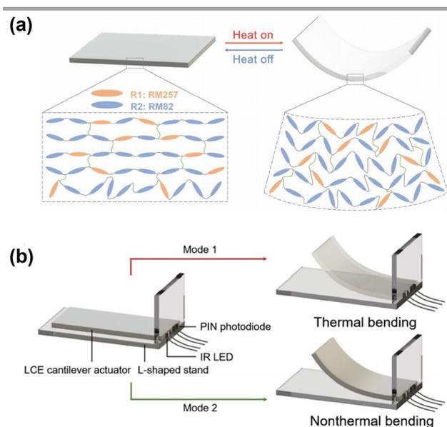
**Figure 9** Thermal bending and optomechanical self-sensing of DLP-printed LCE actuators. a) Chemical composition and principle of thermo-responsive reversible bending in a layered structure. b) Schematic of optoelectronic components and LCE cantilever actuator in two modes (thermal bending and nonthermal bending). Reproduced with permission.<sup>143</sup> Copyright 2021, American Association for the Advancement of Science.
