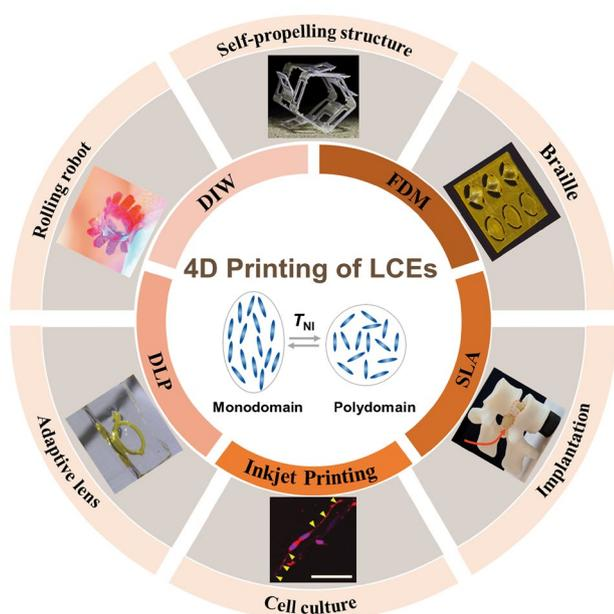
**Figure 2** Representative mechanism, printing methods (DIW, FDM, SLA, DLP, and inkjet printing), and applications of 4D printing of LCEs. (e.g., rolling robot, self-propelling structure, braille, adaptive lens, bone implantations and cell culture.) Reproduced with permission.<sup>66-71</sup> Copyrights 2018, 2019, 2020, 2020, 2020, Wiley-VCH, Copyright 2019, American Association for the Advancement of Science.
