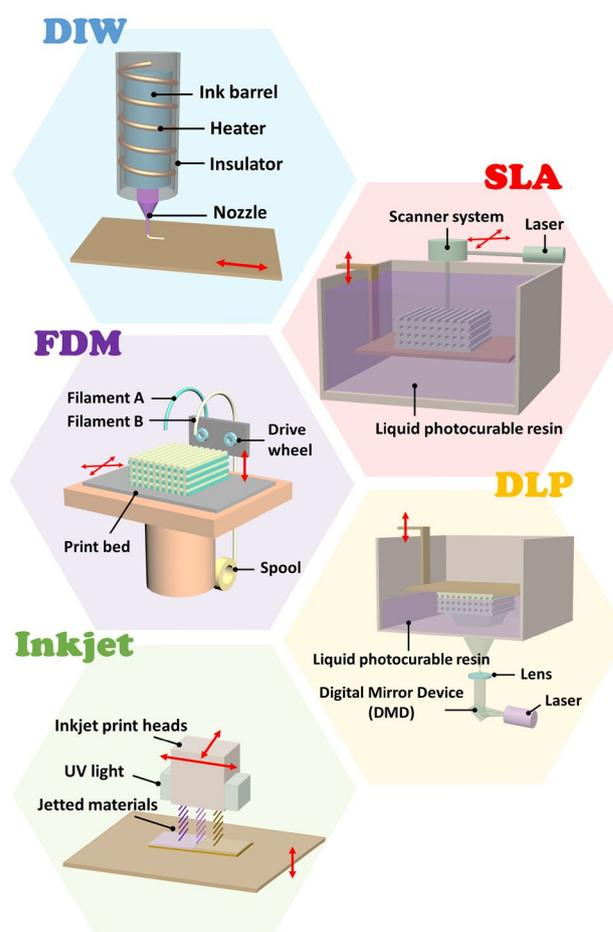
**Figure 6** Schemes illustrating printing techniques for 4D printing of LCEs. Extrusion-based DIW and FDM form 3D projects in a line-by-line and then layer-by-layer manner. Vat photopolymerization-based SLA and DLP can print in sub-micron resolution with high fidelity. SLA employs laser beam and scanner system while DLP relies on digital mirror device (DMD) to achieve dynamic pattern generation. Inkjet printing uses a thermal or piezoelectric actuator to jet materials.
