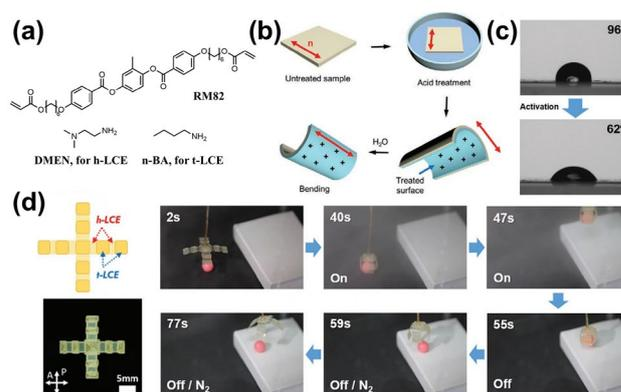
**Figure 13** Humidity-responsive 4D-printed LCEs. a) Chemical composition of h-LCE and t-LCE. b) Schematic of monodomain h-LCE activation by acidic solution (0.1 M HCl) and its bending behavior upon exposure to moisture. c) Contact angles of an h-LCE before and after acid activation. d) LCE soft gripper integrating both h-LCE and t-LCE. Grabbing, transporting, holding, and releasing functions are achieved by humidity control. Reproduced with permission.<sup>193</sup> Copyright 2021, Wiley-VCH.
