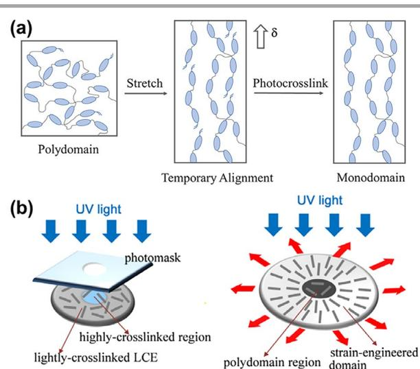
**Figure 4** Mechanical stress-induced alignment. (a) A commonly used two-step alignment of LCE mixtures, which can be temporarily aligned through uniaxial mechanical stretching, and photocrosslink into programmed monodomain. (b) Photomask-assisted inhomogeneous stretching can lead to distinct circular constraints in the LCE sheet. Reproduced with permission.<sup>124</sup> Copyright 2015, Elsevier Ltd.
