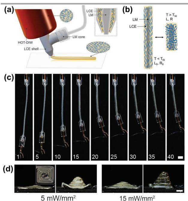
**Figure 12** Liquid metal-enabled electro-responsive 4D-printed LCE actuators. a) Scheme of core-shell iLCE fibers composed of LM core and LCE shell. b) Scheme of iLCE actuation when cycled above and below  $T_{Ni}$ . c) Optical images of electrothermally actuated iLCE fibers with discrete power inputs of 1 and 40  $\text{mW mm}^{-2}$  (scale bars = 5 mm). d) 3D actuation of iLCE spiral structure with closed loop control. Reproduced with permission.<sup>185</sup> Copyright 2021, Wiley-VCH.
