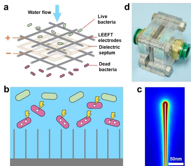
**Figure 1.** Introduction to locally enhanced electric field treatment (LEEFT). **(a)** Schematic of water carrying bacteria through porous electrodes for LEEFT inactivation. **(b-c)** Schematic **(b)** and COMSOL simulation **(c)**, respectively, of lightning-rod effect at the nanowire tip, which enhances the external electric field. **(d)** Optical image of a LEEFT device equipped with the nanowire-modified electrodes.<sup>56</sup>
