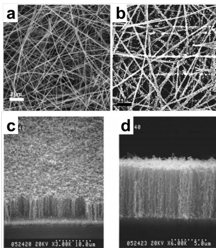
**Figure 7.** Unfavorable nanowire morphology for LEEFT electrodes. (**a & b**) SEM images of pure  $\text{TiO}_2$  (**a**) and  $\text{Ag/TiO}_2$  (**b**) nanofibers. (**c & d**) SEM images showing vertically well-aligned CNTs over a large area (**c**), and in an enlarged and perpendicular view (**d**).<sup>41, 42</sup>
