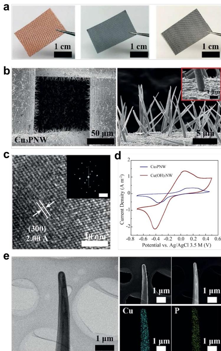
**Figure 4.** Highlights of the Cu<sub>3</sub>PNW-modified electrodes. (a) Optical images of the Cu (substrate), Cu(OH)<sub>2</sub>NW-modified Cu (intermediate), and Cu<sub>3</sub>PNW-modified Cu (product) meshes. (b) SEM images showing Cu<sub>3</sub>PNWs have a diameter of ~500 nm and length of 10 μm, standing vertical to electrode surface. (c) High resolution TEM of the Cu<sub>3</sub>PNW crystal structure.
