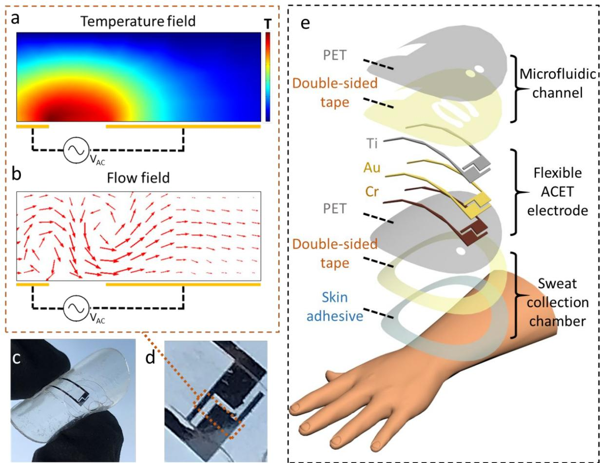
**Fig. 1. Wearable ACET actuation:** a,b) Conceptual illustrations of the ACET-induced temperature (a) and flow field (b) profiles, generated by an asymmetric coplanar pair of electrodes. c,d) Epidermal microfluidic device with an embedded ACET electrode pair. e) Exploded view of the epidermal microfluidic device structure.
