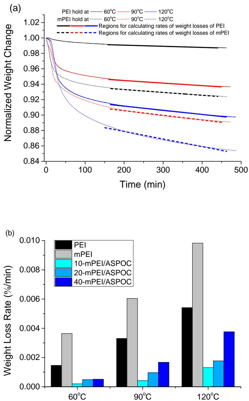
**Figure 6.** (a) Thermal stability of the PEI and mPEI at 60 °C, 90 °C, and 120 °C, and corresponding regions for calculating rates of weight losses. (b) rate of weight loss of the composite samples, PEI and mPEI under 60 °C, 90 °C, and 120 °C.
