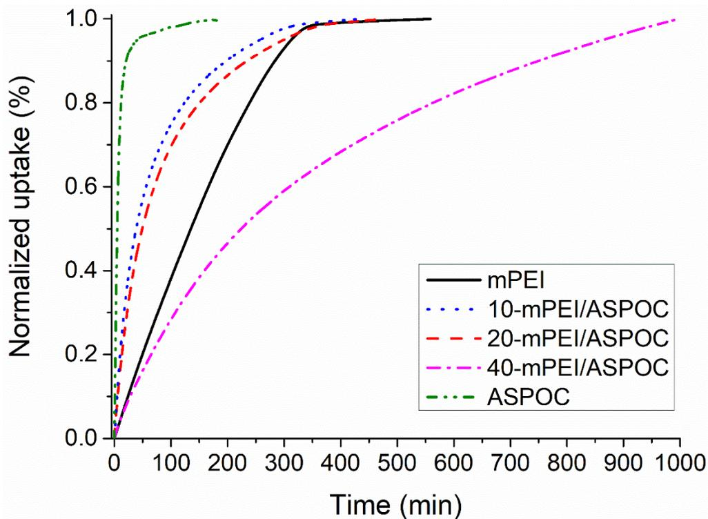
**Figure 5.** SO<sub>2</sub> adsorption kinetics in pure mPEI, ASPOC and mPEI/ASPOC composites at 25°C
