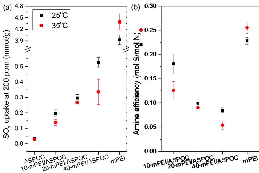
**Figure 4.** (a) SO<sub>2</sub> uptakes of pure ASPOC, mPEI and mPEI/ASPOC composites at 25°C and 35 °C; and (b) corresponding amine efficiencies. SO<sub>2</sub> uptake capacities for 40-mPEI/ASPOC are determined at 1000 min of adsorption as the uptake is slow and did not reach pseudo equilibrium.
