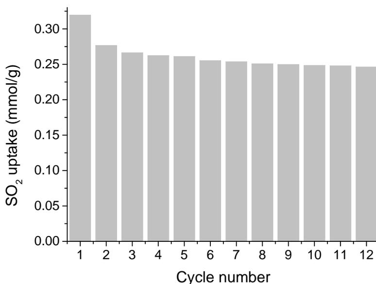
**Figure 8.** Cyclic SO<sub>2</sub> uptake performance of 20-mPEI/ASPOC with a sorption temperature of 25°C and a desorption temperature of 60°C.
