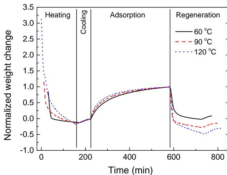
**Figure 7.** Weight change profiles of 20-mPEI/ASPOC during activation-adsorption-regeneration cycle under 60 °C, 90 °C, and 120 °C. The data are normalized by sample dry weight.
