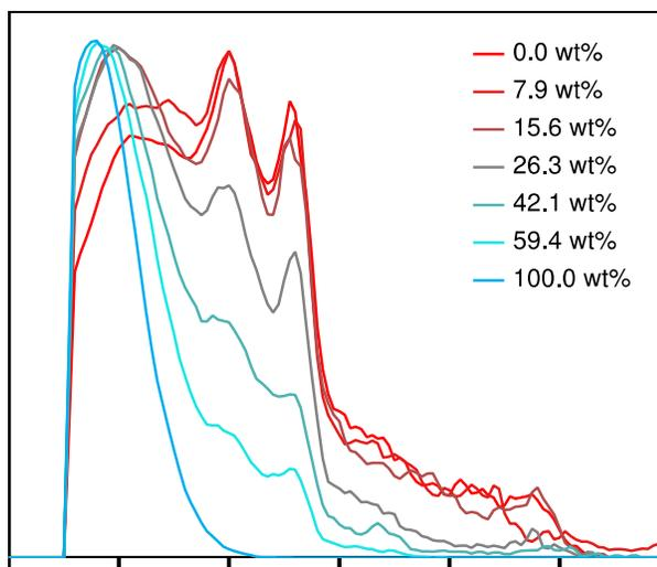
**Figure 2.** Pore size distribution (PSD) of mPEI and ASPOC composites as a function of mPEI loading.
