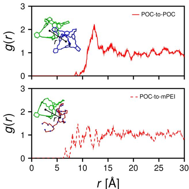
**Figure 3.** Partial radial distribution functions  $g(r)$  of the distance,  $r$ , which denotes the distance between the center-of-mass position between ASPOC molecules (top) and between 26.3% wt mPEI composites (bottom). The images in the inset depict the different definitions of  $r$ .
