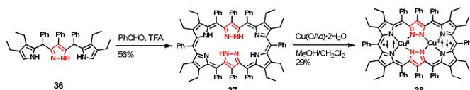
Scheme 3 Synthesis of expanded porphyrin **37** and its dicopper complex **38**.
