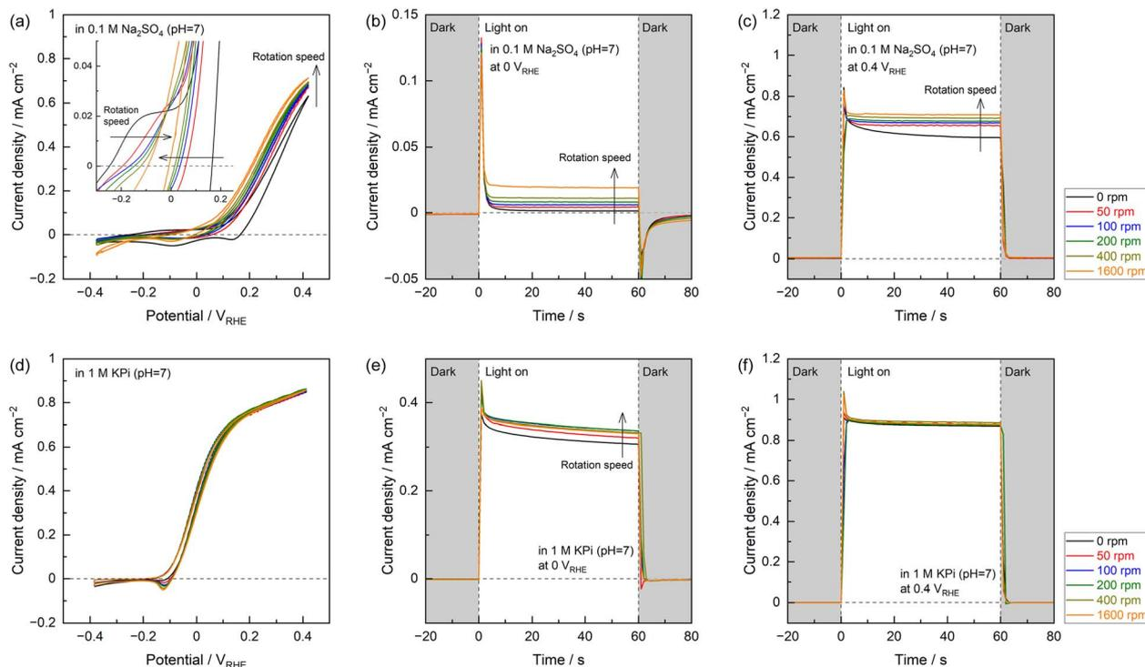
Fig. 2 (a) CV data and current–time curves acquired at applied potentials of (b) 0 and (c)  $0.4 V_{\text{RHE}}$  with a rotating Nb:STO disk electrode at various rotation rates in a  $0.1 \text{ M Na}_2\text{SO}_4$  electrolyte and (d–f) the same plots obtained in a  $1 \text{ M KPi}$  electrolyte. A  $365 \text{ nm}$  LED light source was used.
