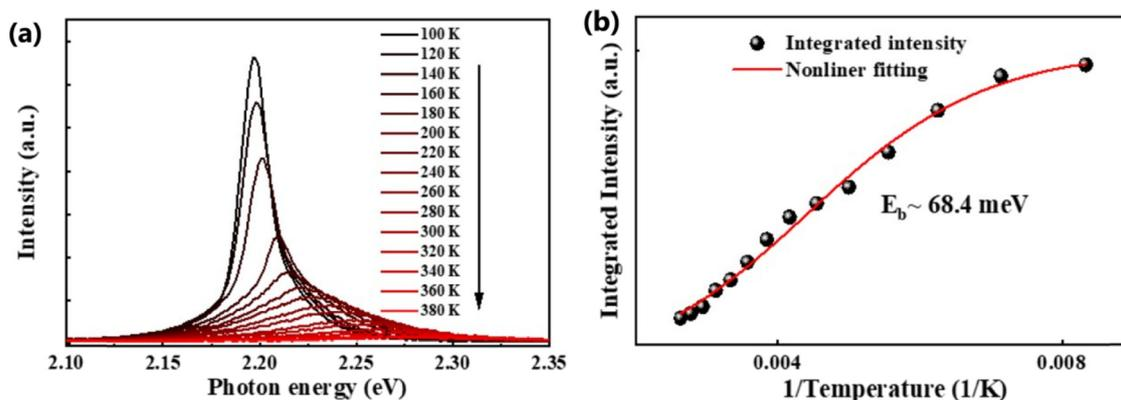
Fig. 3 (a) Temperature-dependent PL spectra of the FAPbBr<sub>3</sub> NCs from 100 K to 380 K. (b) The integrated PL intensity with respect to temperature; the red line corresponds to nonlinear fitting. Adapted from ref. 137, Copyright 2019, American Chemical Society.
