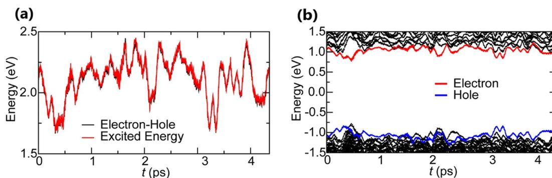
Fig. 5 (a) Time evolution of the many-body electronic excitation energy, including excitonic binding (red), in a  $2 \times 2 \times 2$  supercell nonadiabatic quantum molecular dynamics (NAQMD) simulation, along with compared energy difference between the electron and hole (black). (b) Time evolution of KS eigen energies, with the KS states that mostly contribute to the quasi-electron and quasi-hole shown in red and blue, respectively. Adapted from ref. 85, Copyright 2016, Springer Nature.
