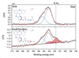
**Fig. 1** S2*p* XPS region acquired on the **RadESAc** bulk sample (top) and on the **RadESAc@Au** monolayer deposited on Au(111). The dashed line highlights the position of the component attributed to the formation of S-Au bond.
