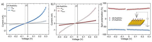
Fig. 3 //v curves acquired on (a) (P)-RadESAc@Au and on (b) (M)-RadESAc@Au applying either positive or negative magnetic field equal to ±0.5 T. Vertical dashed lines indicate the zero-current bias voltage. (c) Spin polarization percentage extracted from the corresponding I/V curves for both the enantiomers at room temperature. Error bars are presented for each point. Inset: Scheme of the experimental setup of mc-AFM.
