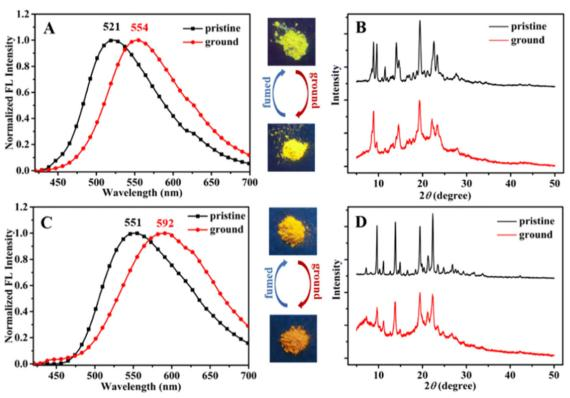
Fig. 7 Fluorescence spectra (A) and (C) and powder XRD patterns (B) and (D) of compounds **9** and **11**, respectively. Inset: Fluorescence images under 365 nm UV light. Reproduced with permission from ref. 75. Copyright 2022 Royal Society of Chemistry.
