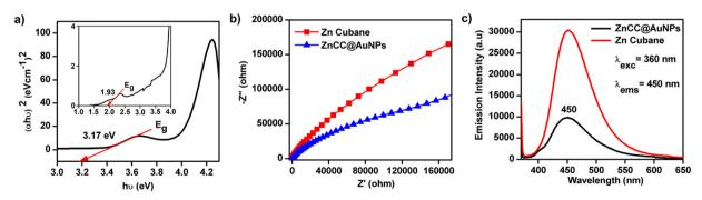
Fig. 6 (a) Tauc plot of ZnCC@AuNPs showing the band gap  $E_{\rm g}$  (inset: magnified view of the Tauc plot showing a weak band due to LSPR), (b) EIS of Zn cubane and ZnCC@AuNPs, and (c) photoluminescence response of Zn(II) cubane and ZnCC@AuNPs
