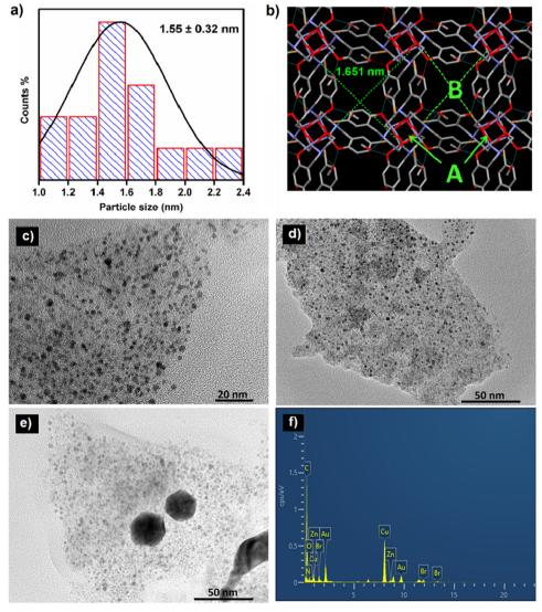
Fig. 4 (a) Particle size distribution of AuNPs, (b) crystal image of the Zn cubane template showing void 'B' of size 1.651 nm, (c)-(e) HR-TEM images of ZnCC@AuNPs at different mass loadings, and (f) elemental distribution analysis of ZnCC@AuNPs.
