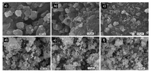
Fig. 3 (a)-(c) FE-SEM images of Zn cubane and (d)-(f) SEM images of ZnCC@AuNPs
