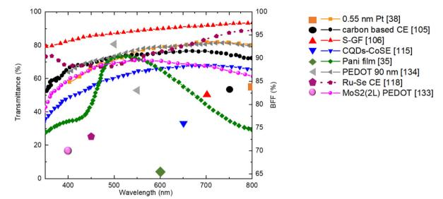
Transmittance (right Y axis) and BFF (left Y axis) of semi-transparent CEs which gave the best performance in terms of PCE and BFF (> 65%).
