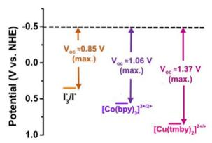
Fig. 7 Potential of for  $I_3^-/I^-$ ,  $[Co(bpy)]^{3+/2+}$  and  $[Cu(tmby)_2]^{2+/+}$  and maximum V<sub>OC</sub> limit
