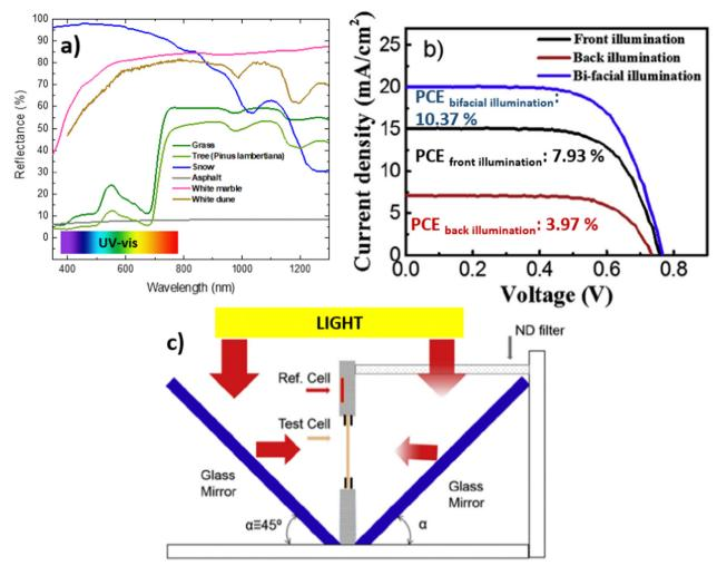
Fig. 3 (a) Reflectance data for different surface materials downloaded from Ecostress Spectral Library provided by the NASA Jet Propulsion Laboratory.<sup>65</sup> (b) J-V curves of a solid state BFDSC device by a back illumination, front illumination and bi-facial illumination (modified from ref. 68). (c) Schematic illustration of the light-splitting design in the bifacial cell tester, with simulated sunlight irradiating on both sides of the cell (modified image from ref. 68).
