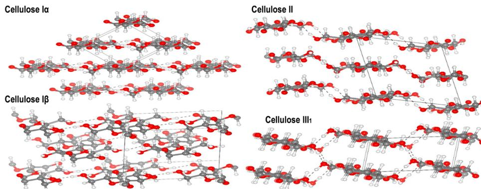
Fig. 12 Refined crystal structures of cellulose allomorphs I $\alpha$ , I $\beta$ , II, and III1 are shown, with carbon, oxygen, and hydrogen atoms depicted as gray, red, and white spheres, respectively. Hydrogen bonds are indicated by dashed lines. Reproduced with permission from ref. 269 Copyright © 2020 Elsevier.
