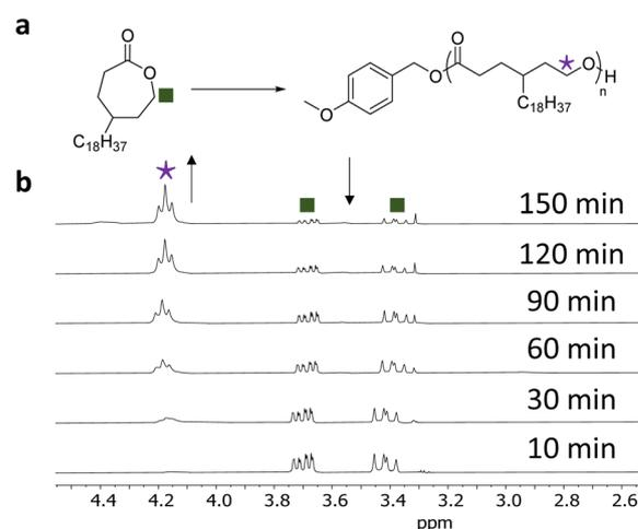
**Fig. 1** (a) ROP of  $\gamma\text{C}_{18}\text{CL}$  using DPP (10 mol%), 4-methoxybenzyl alcohol ( $[\text{M}]_0/[\text{I}]_0 = 50$ ), benzene- $d_6$ . (b) Stacked  $^1\text{H}$  NMR spectra (benzene- $d_6$ , 300 MHz) during ROP of  $\gamma\text{C}_{18}\text{CL}$  showing the  $\text{CH}_2\text{OC}=\text{O}$  monomer resonance between  $\delta = 3.37\text{--}3.70$  ppm and  $\text{CH}_2\text{OC}=\text{O}$  polymer resonance at  $\delta = 4.2$  ppm.
