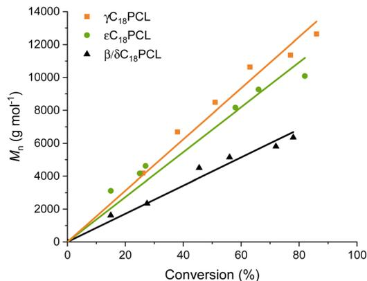
**Fig. 2** Number-average molar mass ( $M_n$ ) plotted against monomer conversion for the ROP of  $\gamma$ C<sub>18</sub>CL,  $\epsilon$ C<sub>18</sub>CL and  $\beta/\delta$ C<sub>18</sub>CL isomers using DPP (10 mol%) and 4-methoxybenzyl alcohol as initiator ( $[M]_0/[I]_0 = 50$ ). Number-average molar mass ( $M_n$ ) determined by SEC analysis in CHCl<sub>3</sub> (0.5% NEt<sub>3</sub>), calibrated against polystyrene standards.
