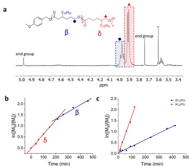
**Fig. 3** (a) <sup>1</sup>H NMR spectrum (CDCl<sub>3</sub>, 400 MHz) of  $\beta$  and  $\delta$ C<sub>18</sub>PCL. \* = MeOH. (b) Semi-logarithmic kinetic plot time for the ROP of  $\beta/\delta$ C<sub>18</sub>CL isomers. (c) Resolved semi-logarithmic kinetic plot for the ROP of  $\beta/\delta$ C<sub>18</sub>CL isomers.  $[M]_0 = 0.5$  M (calculated by NMR spectroscopy based on a starting ratio of  $\beta$  isomer :  $\delta$  isomer = 1 : 1).
