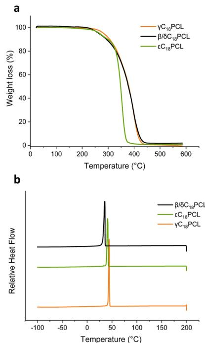
**Fig. 5** (a) Thermogravimetric analysis (TGA) of  $\gamma\text{C}_{18}\text{PCL}$ ,  $\epsilon\text{C}_{18}\text{PCL}$  and  $\beta/\delta\text{C}_{18}\text{PCL}$  isomers. Analytical data of the analysed polymers is summarised in Table 1. (b) Differential scanning calorimetry (DSC) for 2<sup>nd</sup> cooling cycle (200 to  $-100$  °C,  $10$  °C  $\text{min}^{-1}$ ) showing crystallisation and melting temperature of the polymers.
