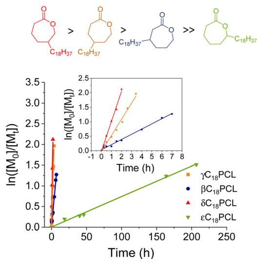
**Fig. 4** Semi-logarithmic kinetic plot for ROP of  $\epsilon\text{C}_{18}\text{CL}$ ,  $\gamma\text{C}_{18}\text{CL}$  and  $\beta/\delta\text{C}_{18}\text{CL}$  isomers using DPP (10 mol%) and 4-methoxybenzyl alcohol as initiator ( $[\text{M}]_0/[\text{I}]_0 = 50$ ).  $\ln([\text{M}]_0/[\text{M}]_t)$  was determined by  $^1\text{H}$  NMR spectroscopy.
