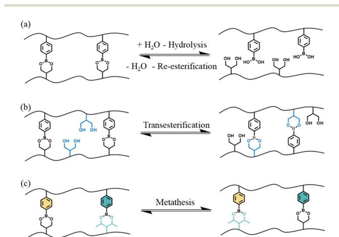
**Fig. 1** Three possible exchange mechanisms of boronic esters: (a) hydrolysis/re-esterification, (b) transesterification and (c) metathesis. Black lines represent polymer chains of the crosslinked network.
