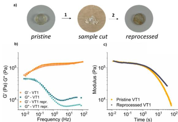
**Fig. 7** (a) Reprocessing of vitrimer network VT1: step 1 consists in cutting in small pieces the pristine vitrimer material. Step 2 refers to the thermal reprocessing at 150 °C for 10 minutes to give the reprocessed material. (b) Storage and loss modulus of pristine and reprocessed VT1. (c) Stress relaxation behaviour of pristine and reprocessed VT1.
