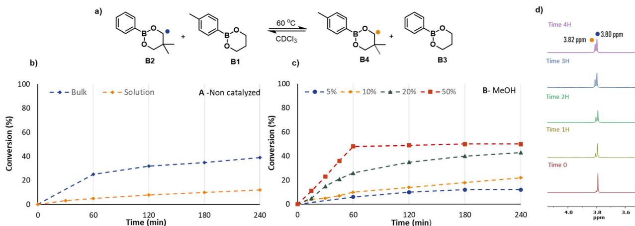
**Fig. 4** (a) Experimental kinetics of the reaction between dioxaborinane **B2** and **B1** at 60 °C for 4 hours. (b) Kinetics of **B2** + **B1** without catalyst in solution (CDCl<sub>3</sub>) and in bulk. (c) Kinetics of **B2** + **B1** in solution with 5, 10, 20 and 50 mol% of MeOH with respect to the dioxaborinanes. (d) Time-dependent <sup>1</sup>H-NMR spectra of the bulk kinetic reaction of the two dioxaborinanes.
