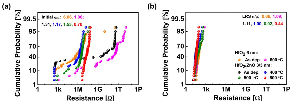
Fig. 4 Distribution and cumulative probability of (a) the initial state during the electroforming process and (b) the low-resistance state (LRS) for single-layer HfO<sub>2</sub> and bilayer HfO<sub>2</sub>/ZnO synaptic devices without and with thermal annealing, where the initial state and LRS were extracted at a read voltage of  $\pm 0.3$  V.
