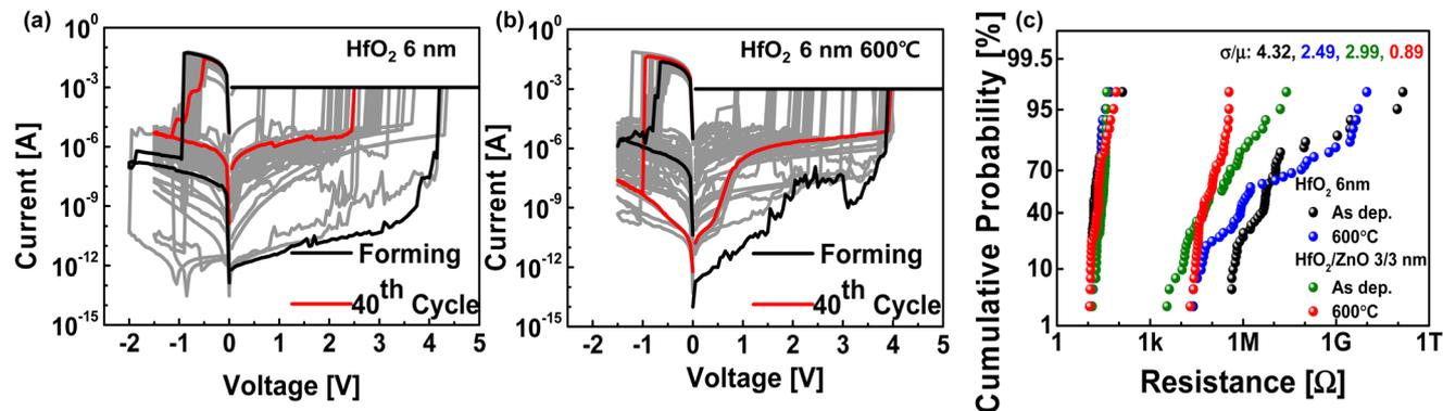
Fig. 7 Typical  $I$ - $V$  switching behavior of 6 nm  $\text{HfO}_2$  (a) without and with thermal annealing (b) at 600 °C for 1 h in an  $\text{N}_2$  ambient compared with that of bilayer  $\text{HfO}_2/\text{ZnO}$  synaptic devices under the same thermal annealing conditions. (c) Distribution and cumulative probability of the HRS and LRS of  $\text{HfO}_2$  (6 nm) and bilayer 3 nm  $\text{HfO}_2/3$  nm  $\text{ZnO}$  synaptic devices without and with thermal annealing.
