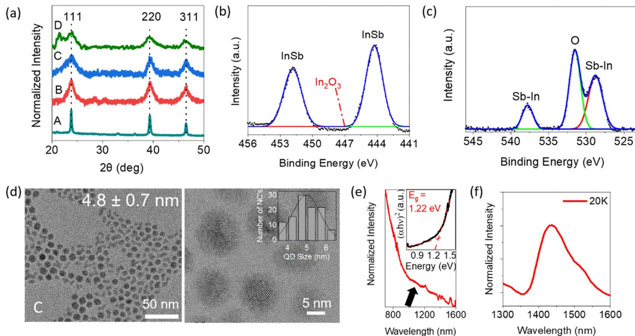
**Fig. 1** (a) Powder XRD patterns of the products prepared with different centrifugation processes; a detailed scheme has been added in Scheme S1 (see ESI†). XPS spectra in (b) In 3d and (c) Sb 3d core levels of sample C, fitted with a Gaussian function. (d) HR-TEM image of sample C with the size distribution profile shown in the inset. (e) Room-temperature NIR absorption spectrum of sample C dispersed in TCE. (f) PL spectra of sample C at a temperature of 20 K.
