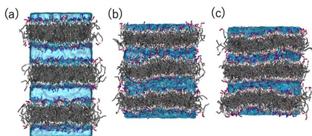
**Fig. 6** Snapshots obtained *via* the MD simulations of Systems (a) 1 (POPC bilayers in aqueous solution), (b) 2 (in 48 vol% ethanol solution), and (c) 3 (in 57 vol% ethanol solution). The POPC molecules are represented as sticks, and the water and ethanol solutions are represented by the cyan color as transparent volume. The color codes of POPC are: NC (choline): blue, PH (phosphate): red, GL (glycerol): silver, EST (ester): white, and CM, CMD2, and CT (hydrocarbons): gray.
