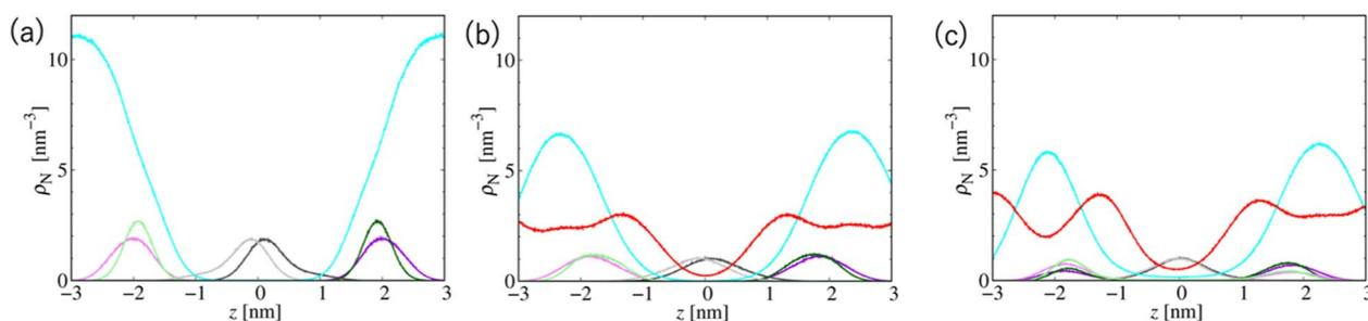
**Fig. 7** Probability density distributions of several selected CG segments along the bilayer normals in Systems (a) 1, (b) 2, and (c) 3. The line colors are WAT: cyan, ETNL: red, CT2 in the oleoyl chain: gray, PH: green, and NC: violet. The latter three lines display darker and lighter color tones in the upper and lower leaflets, respectively.
