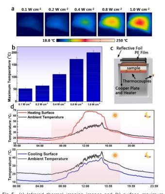
Fig. 5 (a) Infrared thermal imaging images and (b) surface maximum temperature of heating surface irradiated under different light power densities. (c) A diagram of the thermal box was used to quantify the temperature. (d) A continuous twenty-four-hour monitoring of the surface temperature of a dual-mode TMS material and the ambient temperature.
