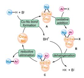
Scheme 1 Proposed catalytic cycle.
