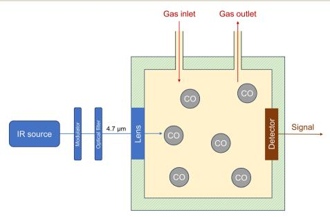
Fig. 1 Principle of photoacoustic spectroscopy (PAS). The specific technical versions of devices<sup>69</sup> may differ from this figure.
