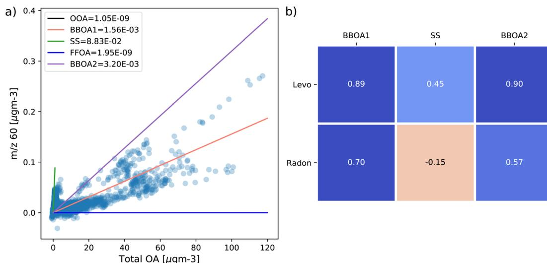
Fig. 4 (a) Concentrations of  $m/z$  60 against concentrations of total OA at COALA, superimposed with lines that use  $f_{60}$  of each factor from the COALA 5-factor PMF solution as their gradient. Values of  $f_{60}$  for each factor are quoted in the legend; (b) Spearman's  $\rho$  coefficients between the concentrations of PMF factors from the COALA 5-factor solution that contain  $m/z$  60 (BBOA1, sea salt, and BBOA2) with levoglucosan (top) and radon (bottom).
