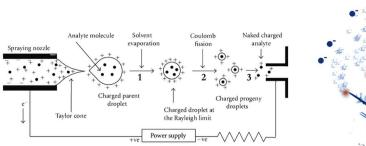
Scheme of electrospray ionization in a mass-spectrometer
