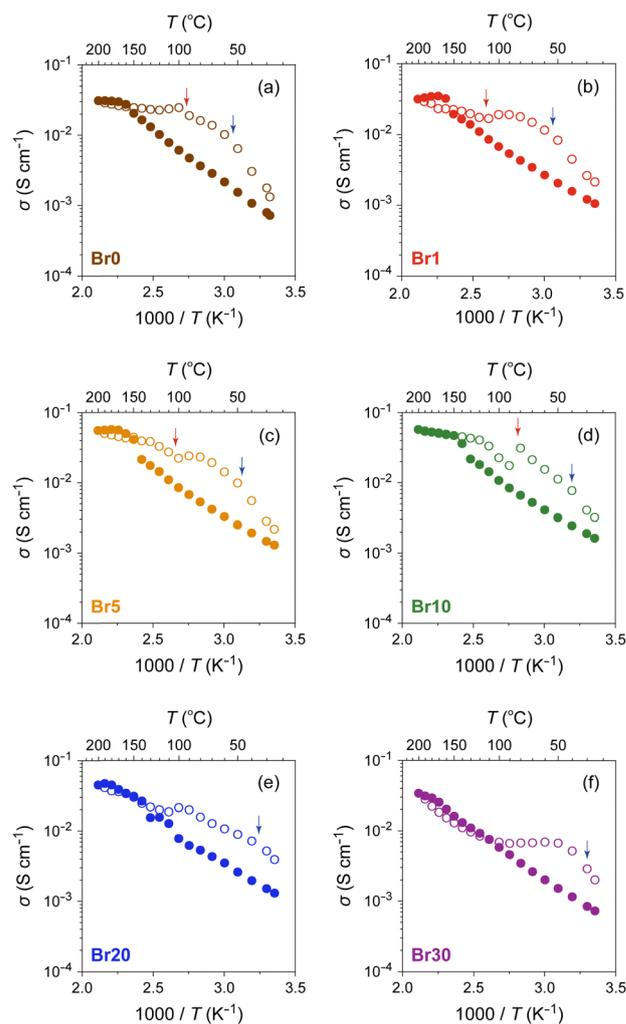
**Fig. 6** Temperature dependence of  $\sigma$  for AgI–AgBr/MPA composites with various AgI : AgBr molar ratios ((a) **Br0**, (b) **Br1**, (c) **Br5**, (d) **Br10**, (e) **Br20**, and (f) **Br30**) in heating (closed circles) and cooling (open circles) processes. The red and blue arrows indicate the onset temperatures of the transition on the high- and low-temperature sides, respectively, in the DSC cooling process (Fig. 3).
