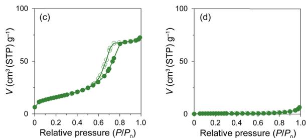
Fig. 2 SEM images and EDS mappings (overlay, Al, Ag, I, and Br) of **Br10** (a) before and (b) after heat treatment.  $N_2$  gas adsorption (closed circles) and desorption (open circles) isotherms of **Br10** (c) before and (d) after heat treatment.
