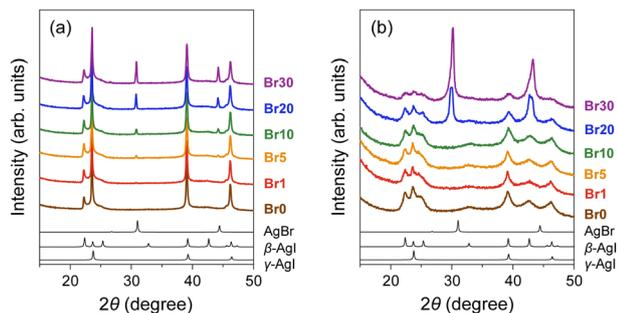
Fig. 1 PXRd patterns of AgI-AgBr/MPA composites with various AgI:AgBr molar ratios (a) before and (b) after heat treatment at 600 °C for 20 h (brown: **Br0**, red: **Br1**, orange: **Br5**, green: **Br10**, blue: **Br20**, purple: **Br30**). Black lines show the simulated patterns of AgBr,  $\beta$ -AgI, and  $\gamma$ -AgI (from the top).
