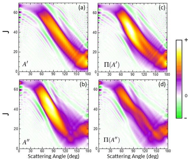
Fig. 5 Generalized quantum deflection functions (GDF) calculated on the  $^3A'$  PES, panel (a), and  $^3A''$ , panel (b), PES for the  $O(^3P) + D_2$  ( $v = 0, j = 0$ ) reaction at  $E_{\text{coll}} = 1.6$  eV. The GDFs resolved in the  $\Pi(A')$  and  $\Pi(A'')$   $\Lambda$ -doublet manifolds are shown in panels (c) and (d), respectively. The color scale is indicated in the figure, with the green contours corresponding to destructive interference ( $Q_r(\theta, J) < 0$ ).
