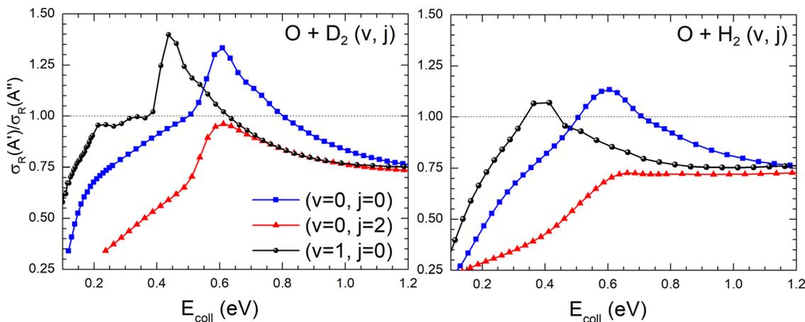
Fig. 9 Comparison of the ratios of the QM cross sections on the  ${}^3A'$  and  ${}^3A''$  PES as a function of  $E_{\text{coll}}$  for the  $O({}^3P) + D_2(v, j)$  (left panel) and  $O({}^3P) + H_2(v, j)$  reactions (right panel).
