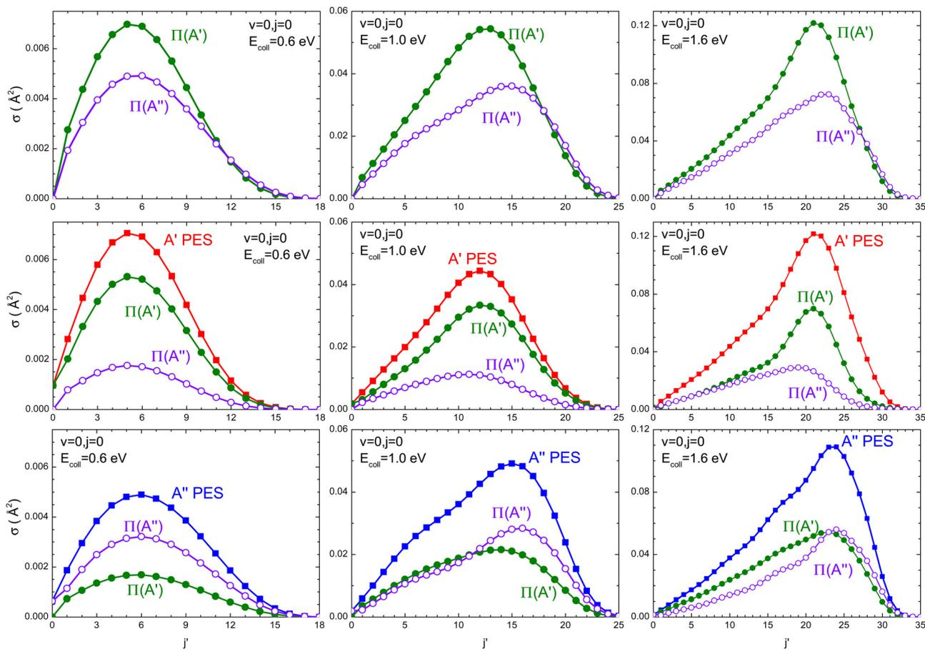
Fig. 4 Top panels: QM rotational distribution (cross section as a function of  $j'$ ) for  $v' = 0$  resolved on the two  $\Lambda$ -doublet manifolds for the  $O(^3P) + D_2$  ( $v = 0, j = 0$ ) reaction at three  $E_{\text{coll}}$ : 0.6 eV, 1.0 eV, and 1.6 eV. Middle panels: QM rotational distribution calculated only on the  ${}^3A'$  PES. Bottom panels: QM rotational distribution calculated only on the  ${}^3A''$  PES.
