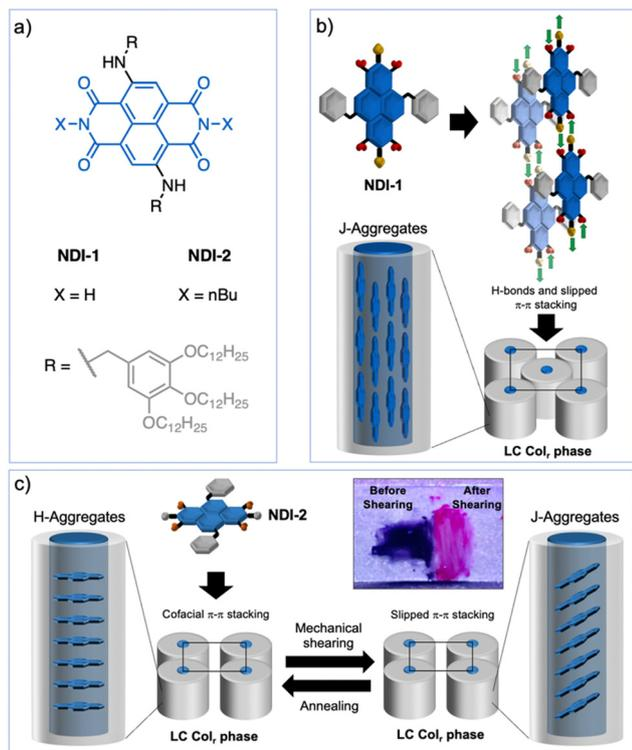
**Fig. 1** (a) Molecular structures of NDI **1** and **2**. (b) Self-assembly behaviour of NDI-**1** into columnar LC J-aggregates driven by H-bonds. (c) Self-assembly properties of NDI-**2** forming columnar LC H-aggregates exhibiting mechano-chromic behaviour caused by a molecular rearrangement in the columnar structure. Inset shows the fluorescence of an NDI-**2** thin film under UV illumination ( $\lambda = 365$  nm) before (left) and after (right) shearing.
