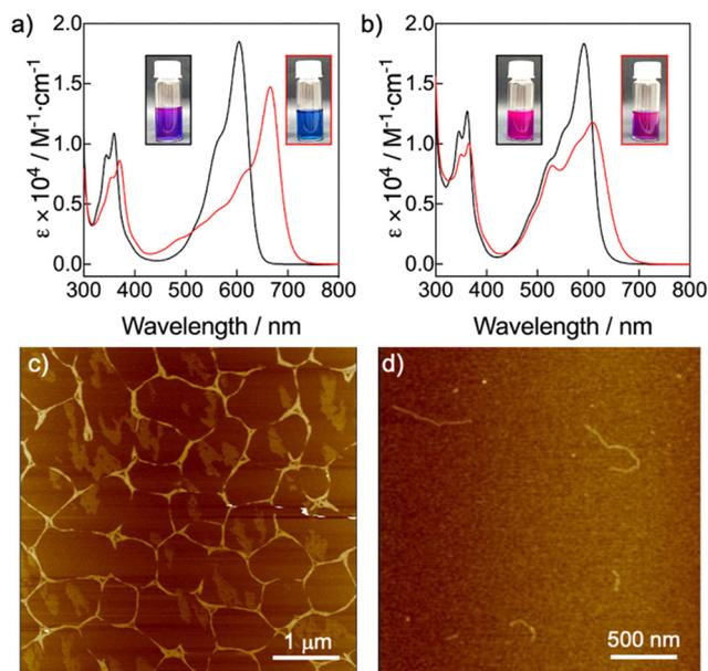
**Fig. 2** UV/vis spectra of (a) NDI-**1** ( $8 \times 10^{-5}$  M) in  $\text{CHCl}_3$  (black line) and in MCH (red line); (b) NDI-**2** ( $5 \times 10^{-5}$  M) in  $\text{CHCl}_3$  (black line) and in MCH (red line). Insets show the corresponding-coloured solutions of the samples. AFM images of (c) NDI-**1** ( $8 \times 10^{-5}$  M) and (d) NDI-**2** J-aggregate ( $5 \times 10^{-5}$  M) spin-coated MCH solutions onto mica substrates.
