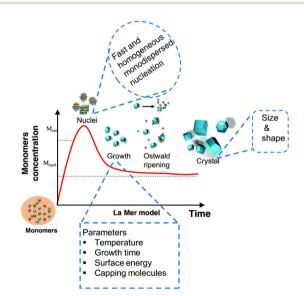
Fig. 3 A graphical representation of the QD formation mechanism. Figure adapted with from ref. 79 with permission from the Royal Society of Chemistry
