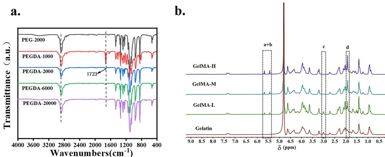
Fig. 2 (a) IR spectra of PEGDA. (b) <sup>1</sup>H NMR of GelMA with different degrees of amino substitution.
