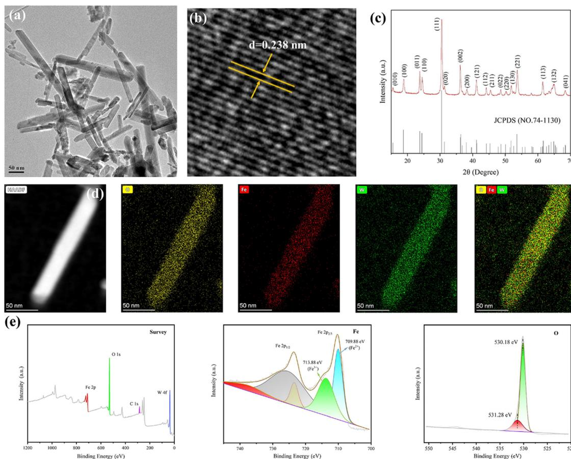
**Fig. 1** Characterization of FeWO<sub>4</sub> nanorods. (a) TEM image, (b) HRTEM image, and (c) XRD pattern of FeWO<sub>4</sub>. (d) Scanning transmission electron microscopy (STEM) images and the corresponding elemental mapping images. (e) Survey XPS spectrum and high-resolution Fe 2p and O 1s spectra of FeWO<sub>4</sub>.
