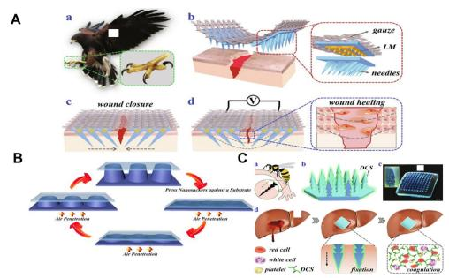
Fig. 5 (A) Schematic illustration of the claw-inspired microneedle patch with liquid metal encapsulation and its wound healing application.<sup>86</sup> Copyright 2021 Elsevier. (B) Schematic diagram of the working principle of the microneedle patch and the equipment process. 91 Copyright 2017 American Chemical Society. (C) Schematic diagram of the preparation of a hemostatic and bionic pagoda microneedle patch. 99 Copyright 2021
