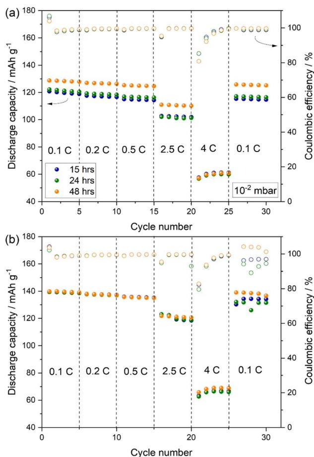
Fig. 9 Rate performance of PW electrodes dried at 170 °C for 15, 24, and 48 hours using a dynamic vacuum of  $10^{-2}$  (a) and  $10^{-3}$  mbar (b). Test conducted at 25 °C using 1 M NaPF<sub>6</sub> in diglyme electrolyte within the 2.0–4.0 V range. (1C =  $140 \text{ mA h g}^{-1}$ ).
