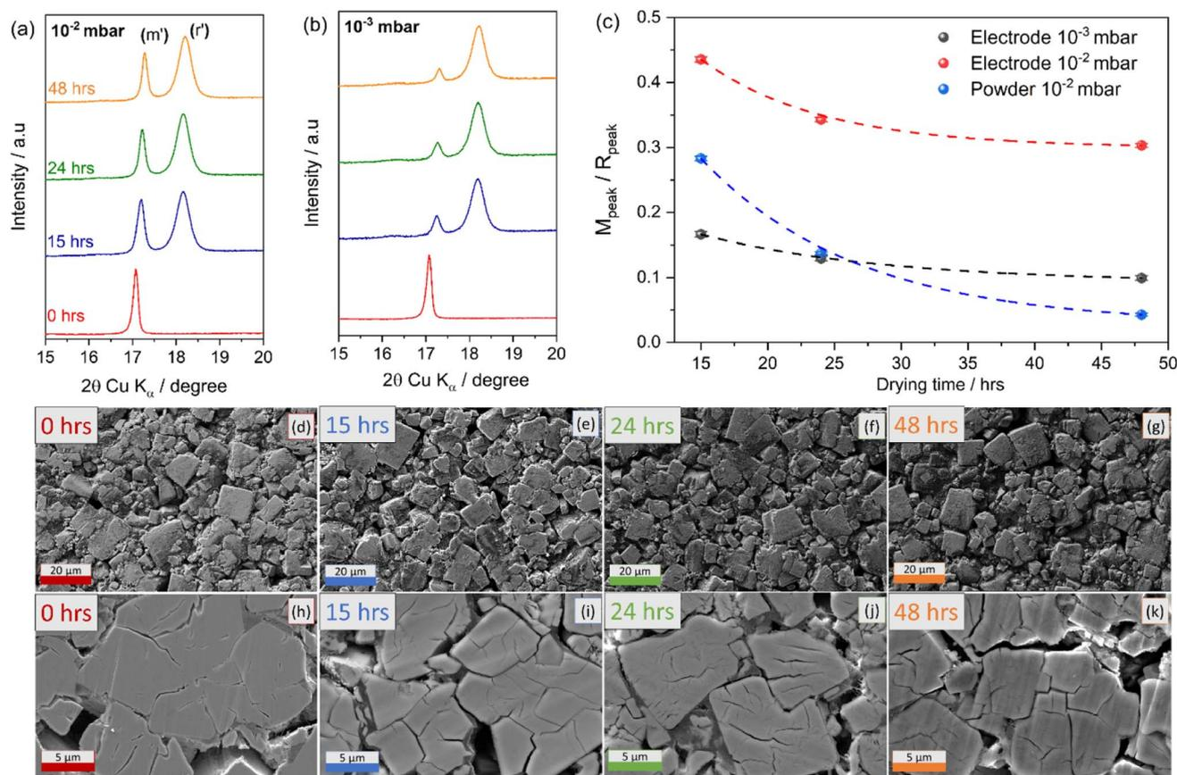
Fig. 5 XRD patterns of PW electrodes dried for 15, 24 and 48 hours at 170 °C under a dynamic vacuum of (a)  $10^{-2}$  mbar, and (b)  $10^{-3}$  mbar. (c) Pseudo-quantitative analysis of monoclinic to rhombohedral transformation and relative phase ratios upon dehydration. Planar (d)–(g) and cross-sectional (h)–(k) SEM images of undried and dried PW electrodes ( $10^{-3}$  mbar).
