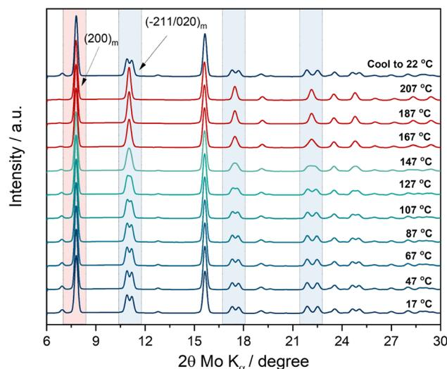
Fig. 1 *In situ* XRD measurement as a function of temperature on pristine PW powder material. Test conducted in transmission mode. Heating rate: 2 °C min<sup>-1</sup>.
