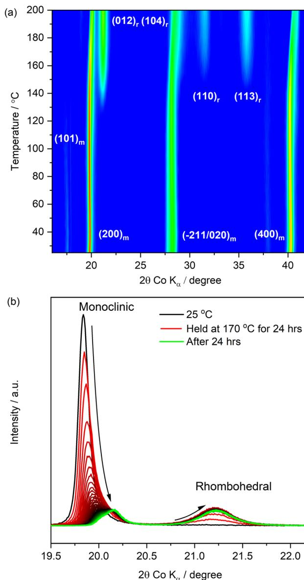
Fig. 4 *In situ* XRD measurement as a function of temperature on pristine PW-based composite electrodes. Test conducted in reflection mode (a) from room temperature (25 °C up to 200 °C, heating rate: 5 °C  $\text{min}^{-1}$ ). (b) From room temperature up to 170 °C with holding step for 24 hours. Both tests conducted under dynamic vacuum ( $10^{-2}$  mbar).
