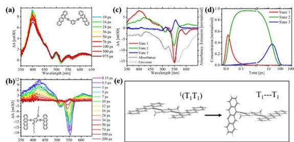
Fig. 5 (a) and (b) TA spectra of dimer **8** (a) and **9** (b) in solution. (c) and (d) Species associated difference spectra (c) and concentration curves (d) from the target analysis of the TA data of dimer **9**. (e) Proposed decoupling of the  $^1(\text{TT})$  state in dimer **10** to give rise to two independent triplets. Reproduced with permission.<sup>99</sup> Copyright 2018, the American Chemical Society.
