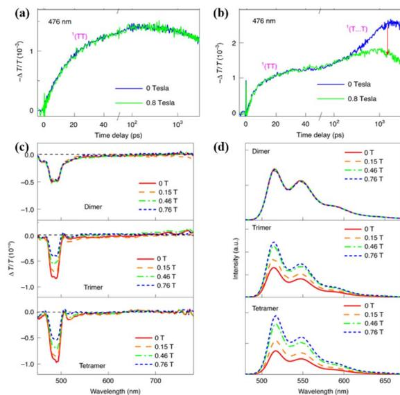
**Fig. 16** (a) and (b) Dynamics of the singlet and triplet states of dimer (a) and trimer (b) with and without application of an external magnetic field of 0.8 T. (c) TA spectra of these oligomers recorded at a time delay of 100 ns, while applying a magnetic field of different magnitudes. (d) Fluorescence spectra of these oligomers with an applied magnetic field of different magnitudes. Reproduced with permission.<sup>173</sup> Copyright 2021, Springer Nature.
