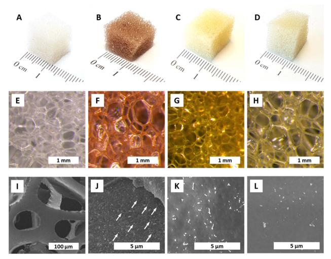
Fig. 1 Aspect and morphology of NPs@PUF. All specimens were synthesized at  $T_R = 120$  °C,  $t_R = 3$  h, and  $[\mathcal{M}^{x+}] = 0.25$  mM. Macroscopic aspect (A-D) and optical micrographs (E-H) of pristine PUF and NPs@PUFs: pristine PUF (A and E), AuNP@PUF (B and F); AgNP@PUF (C and G), PdNP@PUF (D,H). SEM micrographs of pristine PUF(I), and NPs@PUFs: AuNP@PUF (J) with some AuNPs indicated with white arrows; AgNP@PUF (K): and PdNP@PUF (L).
