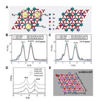
Fig. 3 (A) Structural model of NiFe-LDH nanosheets and NiFe-LDH bulk; R space of the (B) Ni and (C) Fe K-edge EXAFS spectra. <sup>54</sup> Copyright © 2020 Royal Society of Chemistry. (D) R space of Ni K-edge EXAFS spectra. (E) Schematic illustration of the basic unit cell of monolayer NiAl-LDH. <sup>55</sup> Copyright © 2019 Wiley-VCH Verlag GmbH & Co. KGaA, Weinheim.
