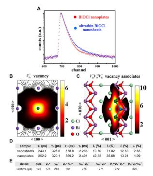
Fig. 8 (A) PAS spectra of ultrathin BiOCl nanosheets and nanoplates. (B and C) Schematic illustrations of trapped positrons of  $V_{Bi}^{'''}$  defects and associated defects  $V_{Bi}^{"'}V_{O}^{"}V_{Bi}^{"}$ . (D) Positron lifetime parameters of ultrathin BiOCl nanosheets and nanoplates. (E) Calculated positron lifetime values of BiOCl. 104 Copyright © 2013 American Chemical Society.
