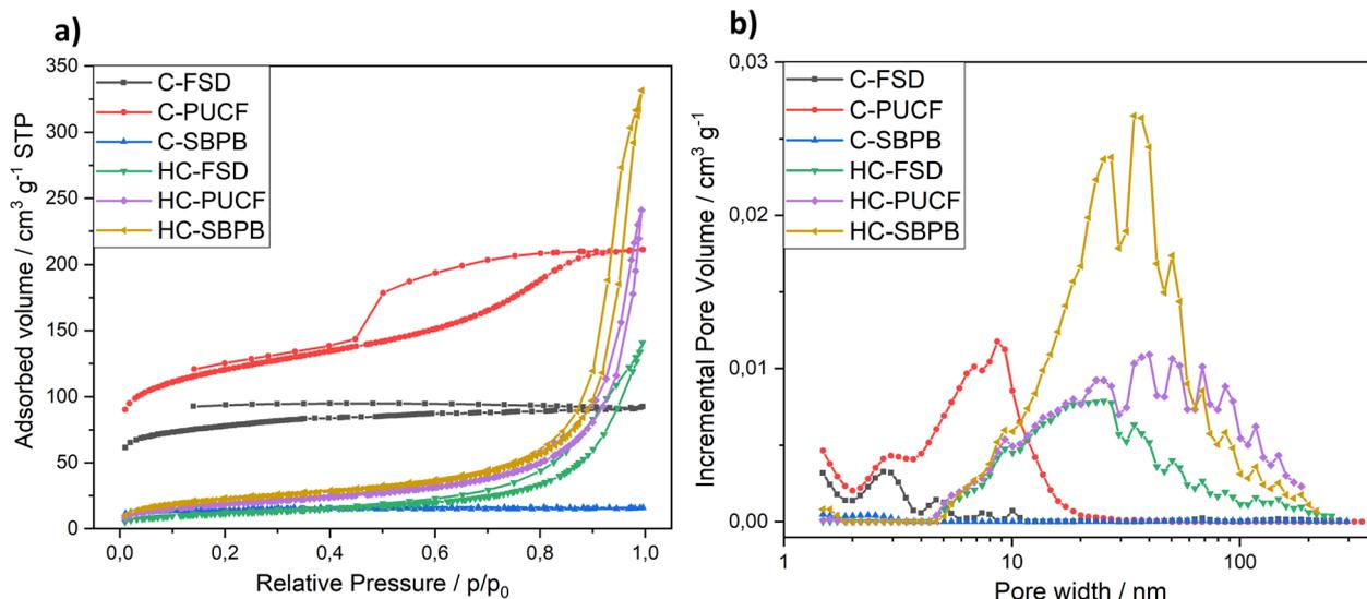
Fig. 7 N<sub>2</sub> adsorption–desorption isotherms (a) and pore size distribution (b) of the samples.
