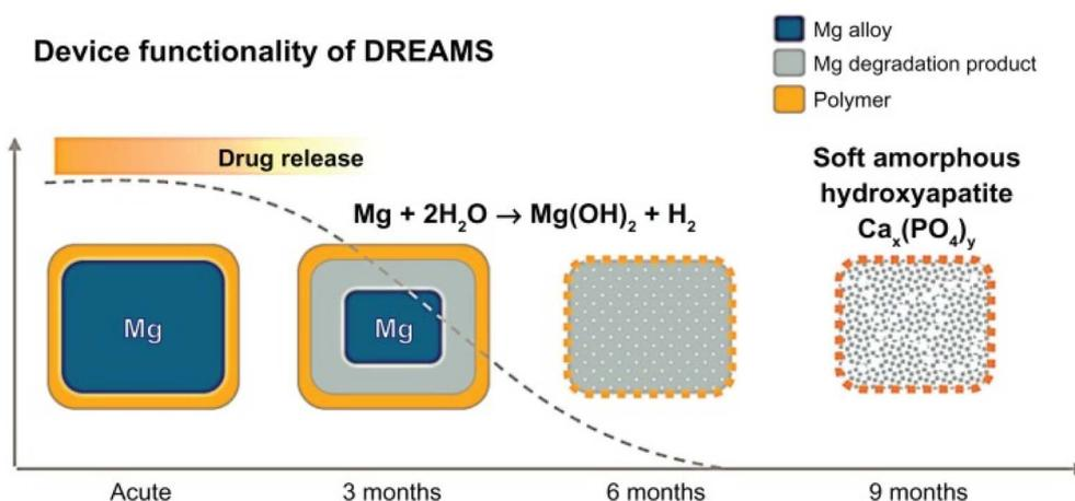
Fig. 4 Degradation model of DREAMS-2 stent.<sup>76</sup>
