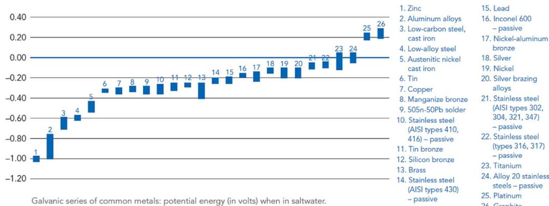
Fig. 23 Galvanic series of metals in saltwater noting electrical potential energy.<sup>238</sup>
