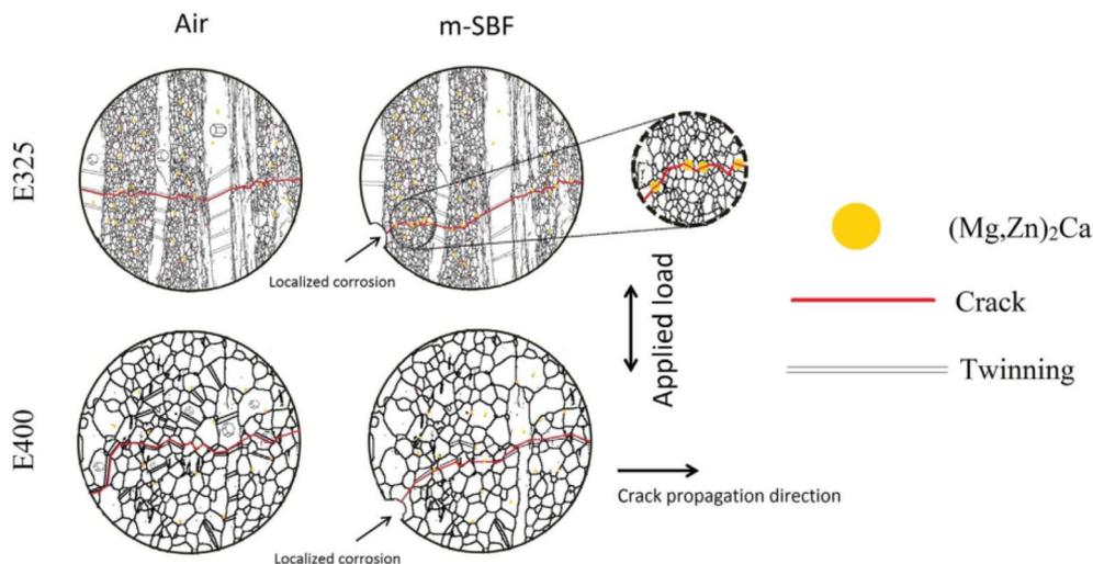
Fig. 12 Schematic diagram of fatigue cracking of ZX10 extruded at 325 °C and 400 °C when tested in air and m-SBF.<sup>126</sup>
