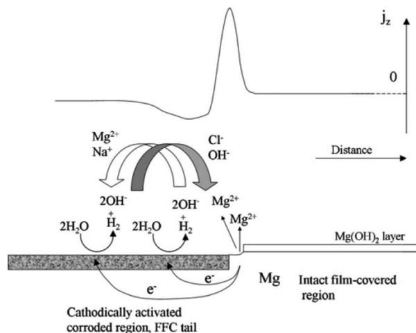
Fig. 9 Schematic representation of the mechanism of filiform corrosion under immersion conditions, showing how the regions of the localised corrosion cell correspond with empirically derived SVET  $j_z$  versus distance profiles.<sup>142</sup>
