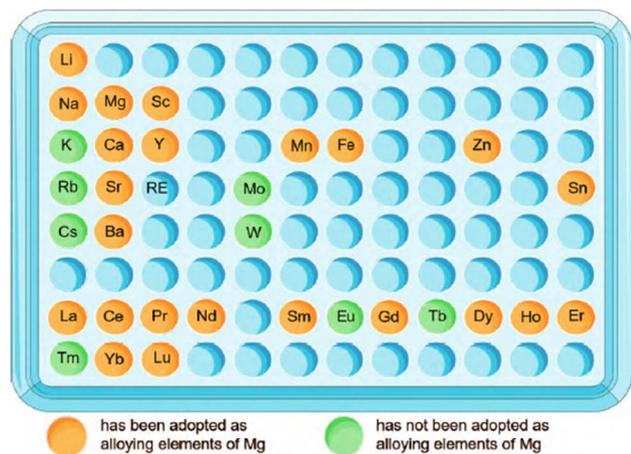
Fig. 17 Suitable elements for magnesium alloying and their applications.<sup>191–193</sup>
