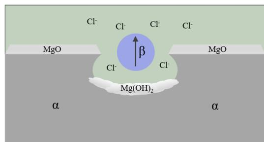
Fig. 7 Schematic of pitting corrosion.<sup>131</sup>
