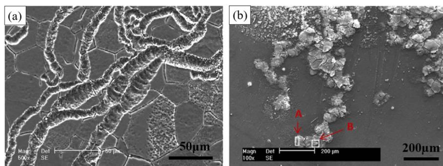
Fig. 10 Typical filamentary corrosion morphologies of Mg–3Zn immersed in 0.01 mol per L NaCl solution for 6 h at different scales (50  $\mu\text{m}$  and 200  $\mu\text{m}$ ).<sup>121</sup>
