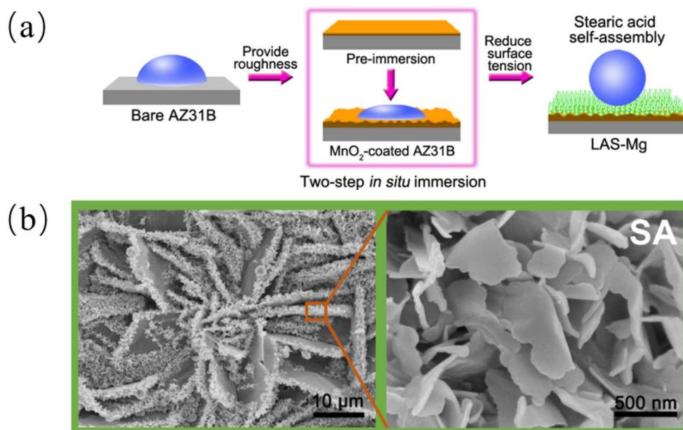
Fig. 27 (a) Schematic illustration of the fabrication process of LAS-Mg. (b) SEM images of LAS-Mg.<sup>263</sup>
