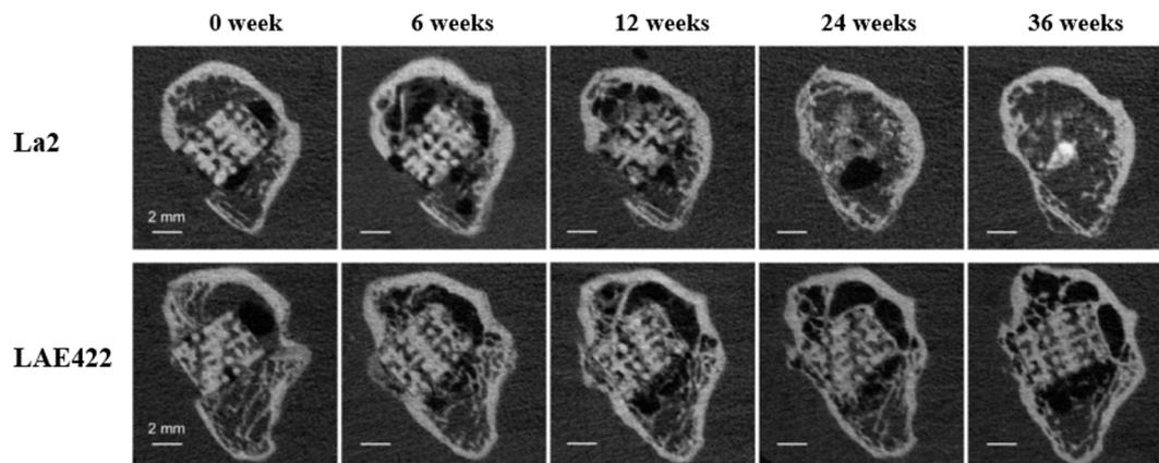
Fig. 3  $\mu$ CT images of longitudinal sections of La2 and LAE422 degradation evolution at 36 weeks.<sup>60</sup>
