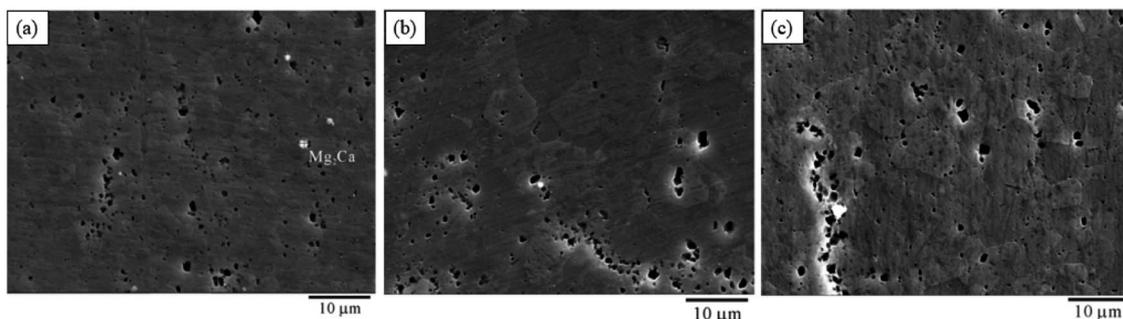
Fig. 18 SEM images of the (a) Mg–0.54Ca alloy; (b) Mg–0.79Ca alloy; (c) Mg–1.35Ca alloy.<sup>198</sup>
