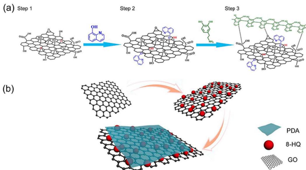
Fig. 24 (a) The synthesis process of sandwich-like GO/8-HQ/PDA structures and (b) schematic illustration of the synthesis of the GO/8-HQ/PDA.<sup>244</sup>
