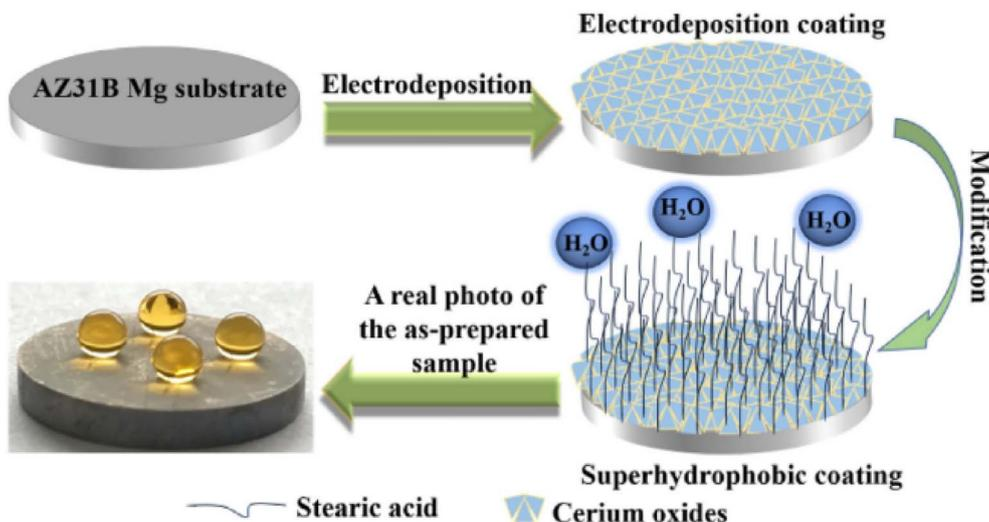
Fig. 28 Schematic diagram of preparation process of the superhydrophobic coating formed on the AZ31B Mg substrate.<sup>266</sup>
