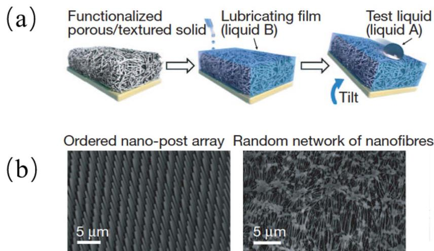
Fig. 30 (a) Schematic diagram of SLIPS assembly process; (b) SEM: an epoxy-resin-based nanofabricated post array (left) and a Teflon-based porous nanofibre network (right).<sup>272</sup>
