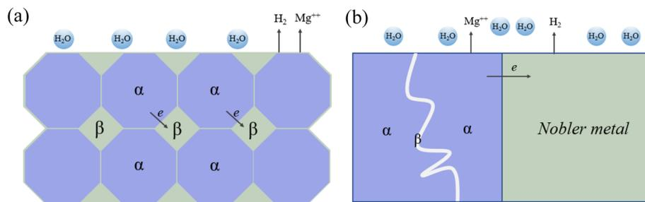
Fig. 6 (a) Schematic of internal micro-galvanic corrosion. (b) External galvanic corrosion.<sup>131</sup>
