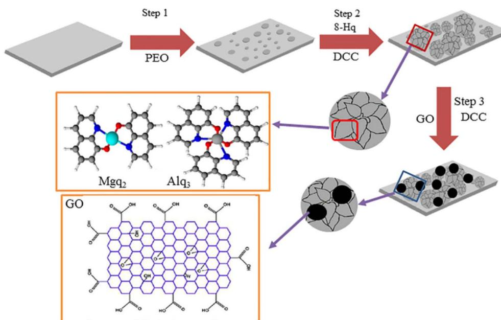
Fig. 25 Schematic diagram of the fabrication steps for GO/8-Hq/IC materials.<sup>248</sup>
