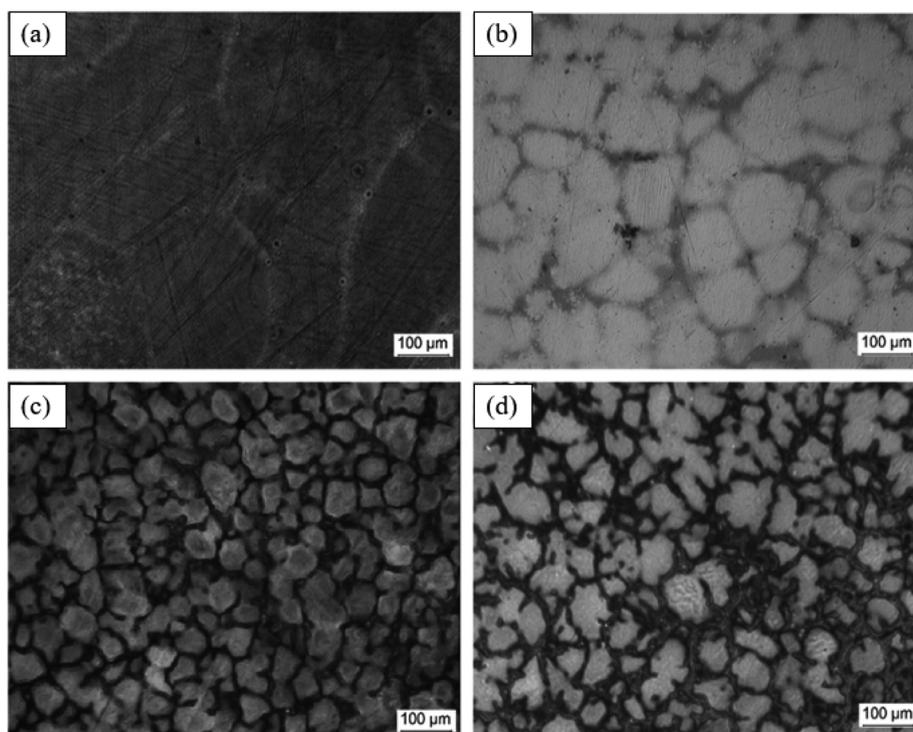
Fig. 20 Optical microstructure changes of Mg–Zn alloys (a) pure Mg, (b) Mg–1Zn, (c) Mg–5Zn and (d) Mg–7Zn.<sup>214</sup>
