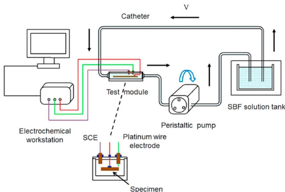
Fig. 16 Schematic diagram of a dynamic flow field test device.<sup>181</sup>
