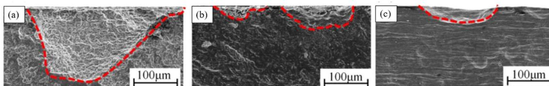
Fig. 15 Pits of ZK60 on the fractures in three solutions. (a) pH 5.2, (b) pH 7.4 and (c) pH 9.0.<sup>176</sup>
