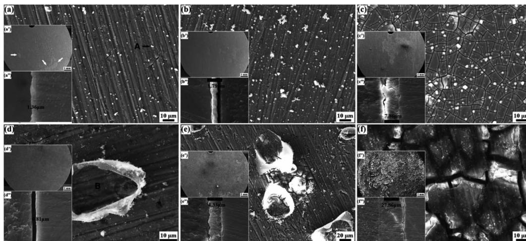
Fig. 13 Surface morphologies of ZK21-0.2Sc alloy after immersion: (a–c) Hank's, (d–f) Hank's + BSA; (a and d) 6 h, (b and e) 12 h, (c and f) 168 h.<sup>163</sup>
