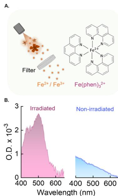
**Fig. 4** Detection of iron ions. (A) Scheme of the purification process and the metal complex used for detecting the presence of released iron ions. Irradiated NFs (or non-irradiated for control) were filtered, and the filtrate was treated with 1,10-Phenanthroline (phen), resulting in the orange-red metal complex [Fe(phen)<sub>3</sub>]<sup>2+</sup>. (B) Extinction spectra obtained from the filtrates of NF dispersions without (blue) and with (magenta) 808 nm irradiation ( $P = 200$  mW).
