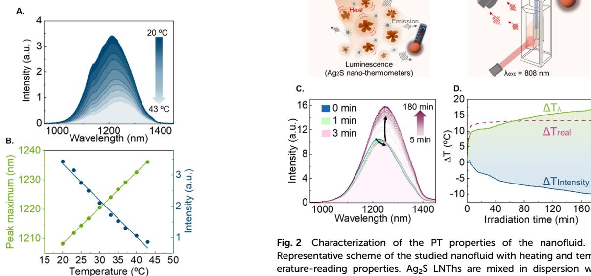
**Fig. 1** Characterization of NIR Ag<sub>2</sub>S nanoparticles as LNTHs. (A) Emission spectra of Ag<sub>2</sub>S LNTHs obtained at different temperatures (from 20 to 43 °C). (B) Multiparametric thermal readouts of the emission spectra of Ag<sub>2</sub>S LNTHs. Intensity and shifting of the peak maximum give inverse linear tendencies with Pearson correlation coefficients close to  $-1$  for the emission intensity and  $1$  for the displacement.
