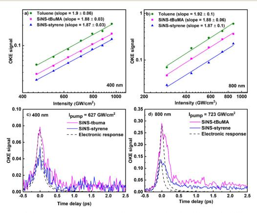
Dependence of the OKE signal on the pump beam intensity and its temporal evolution at (a, c) 400 nm and (b, d) 800 nm.
