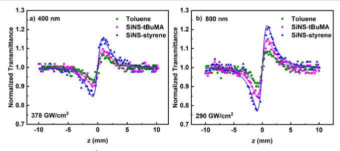
Fig. 7 "Divided" Z-scans of 0.1 mg mL<sup>-1</sup> SiNS-tBuMA and SiNS-styrene dispersions in toluene, under (a) 50 fs, 400 and (b) 70 fs, 800 nm laser excitation.
