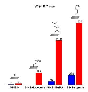
Fig. 9 Third-order nonlinear susceptibility  $\chi^{(3)}$  values of SiNS-H and SiNS-dodecene, SiNS-tBuMA, and SiNS-styrene under 800 nm (red) and 400 (blue) laser excitation, determined by the Z-scan technique. All values refer to a concentration of  $1 \text{ mg mL}^{-1}$ .
