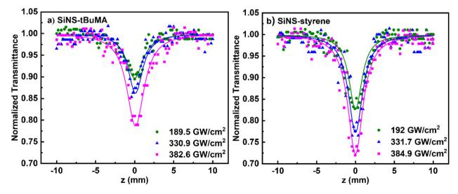
Fig. 5 OA Z-scans of (a) SiNS-tBuMA and (b) SiNS-styrene dispersions under different laser intensities at 800 nm. All dispersions had a linear absorption coefficient  $\alpha_0$  of about 1 cm<sup>-1</sup>.
