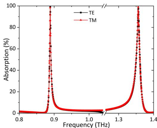
Fig. 2 Absorption spectra of the dual-band metamaterial absorber.
