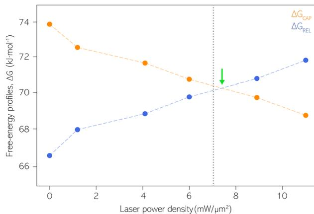
**Fig. 5** Capture and release barriers,  $\Delta G_{\text{REL}}$  and  $\Delta G_{\text{CAP}}$ , respectively, as a function of the laser power density. The dashed lines are a guide to the eye. Vertical dashed line at  $7.1 \text{ mW } \mu\text{m}^{-2}$  indicates the transition where  $K_{\text{ASS}}$  becomes larger than  $K_{\text{DIS}}$  according to Fig. 4. Green arrow indicates the intersection point between  $\Delta G_{\text{REL}}$  and  $\Delta G_{\text{CAP}}$  trends.
