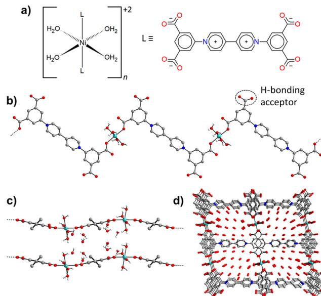
**Fig. 1** Crystal structure of Ni-ZW-MOF. a) Octahedral coordination environment of  $\text{Ni}^{2+}$  cations with L representing the ZW ligand dcpb; 1D zigzag chains shown along the crystallographic b) *b*-axis and c) *c*-axis; and d) packing diagram along the crystallographic *b*-axis. Aromatic hydrogens and disorder are omitted for clarity; grey-carbon, blue-nitrogen, red-oxygen, cyan-nickel.
