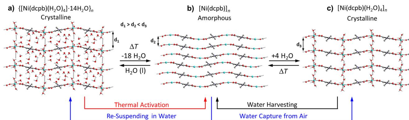
**Fig. 3** Schematic representation of structural changes during thermal activation, water capturing and water harvesting of Ni-ZW-MOF shown along the crystallographic  $c$ -axis. Aromatic hydrogens and disorder are omitted for clarity; dashed lines represent H-bonding; grey-carbon, blue-nitrogen, red-oxygen, cyan-nickel.
