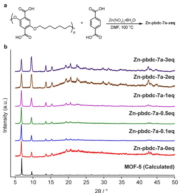
**Fig. 2** Synthesis of mixed ligand polyMOF **Zn-pbdc-7a-xeq**, polyMOFs formed from **pbdc-7a** and *x* equivalents of free H<sub>2</sub>bdc (a) and powder X-ray diffractogram (b) of **Zn-pbdc-7a-xeq** with varying equivalents of free H<sub>2</sub>bdc used in the synthesis.
