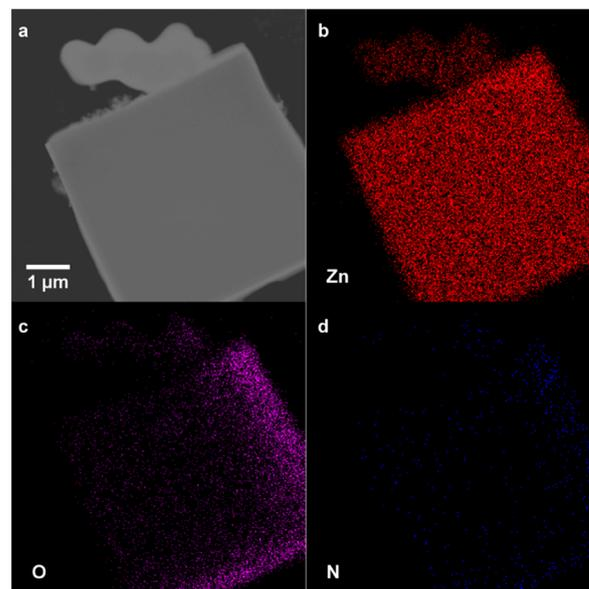
**Fig. 3** (a) TEM image of **Zn-pbdc-7a-2eq-NH<sub>2</sub>** and (b), Zn (c) O, (d) N EDX elemental mapping of **Zn-pbdc-7a-2eq-NH<sub>2</sub>**, indicating incorporation of free bdc-NH<sub>2</sub> ligand into polyMOF lattice.
