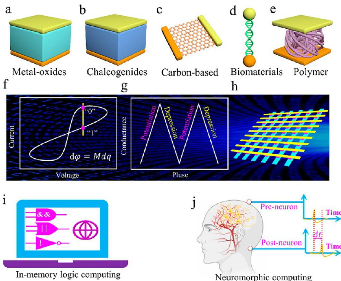
**Fig. 18** Schematic representation of the memristor with various materials, in (a)–(e). (f) Standard voltammetry test with the cyclic  $I$ – $V$  characteristic. (g) Conductance evolution under pulse excitation (voltage or current), simulating the potentiation and depression of biological synapses. (h) Crossbar-structured integrated memristor device schematic diagram. (i) Diagram showing the in-memory logic computing system. (j) Diagram showing the neuromorphic computing system.<sup>255</sup>
