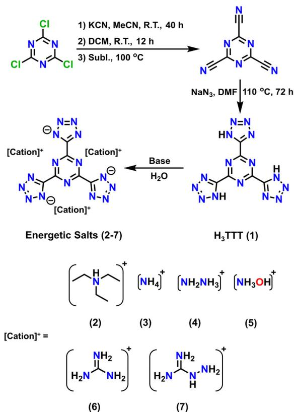
**Scheme 1** Synthetic pathway for the synthesis of 2,4,6-tris(1H-tetrazol-5-yl)-1,3,5-triazine ( $H_3TTT$ , **1**) and its energetic salts (**2-7**). Reagents and conditions are indicated in the scheme.
