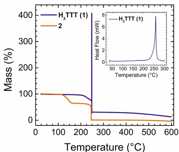
Fig. 3 Thermogravimetric analysis (TGA) of compounds 1 and 2, performed using a temperature ramp of  $10\text{ °C min}^{-1}$ . The significant increase in mass percent observed at 247 °C in 1 is associated with the detonation of the material. (inset) Differential scanning calorimetry (DSC) of 1, also performed at  $10\text{ °C min}^{-1}$ .
