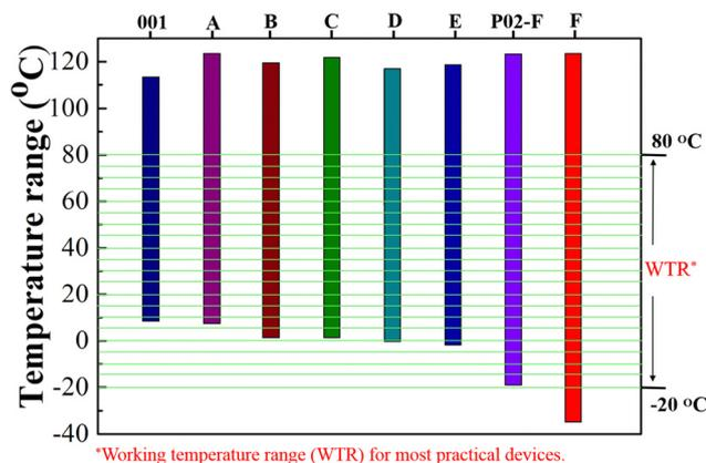
Fig. 4 Effect of target compounds on the temperature range of LC mixtures. Each of five compounds **4TV**, **4FTV**, **4TFV**, **4FTFV** and **2TFV** (15 wt%) was dissolved in LC mixture **001**, yielding new LC mixtures **A**, **B**, **C**, **D** and **E**. Compound **2TFV** (15 wt%) was dissolved in the LC mixture **P02-F**, yielding new LC mixture **F**.
