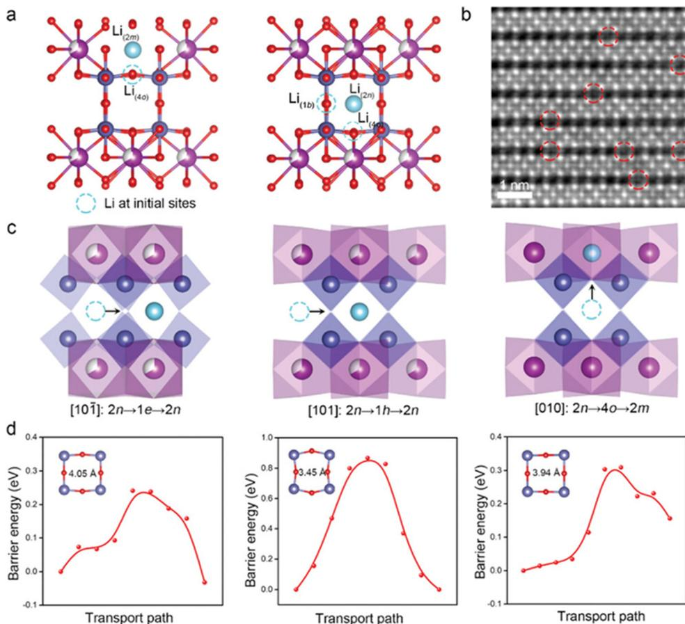
Fig. 7  $\text{Li}^+$  insertion point of CNO calculated by DFT (a). The iDPC image along the [101] direction after charging (b). The  $\text{Li}^+$  migration pathway (c) and the energy profile (d).<sup>87</sup> Copyright © 2022 Wiley VCH.
