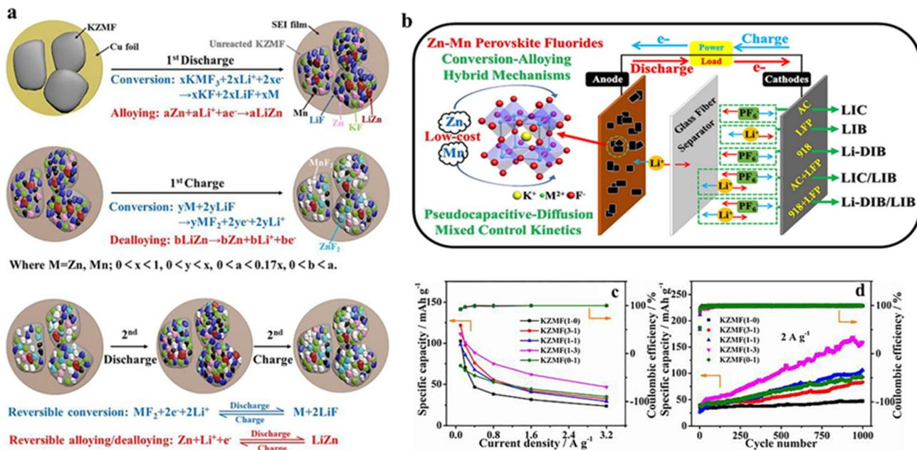
Fig. 5 Reaction mechanism of the KZMF electrode (a). Schematic diagram of potential applications of KZMF for Li<sup>+</sup> storage (b). Specific capacity of KZMF (c) and cycling performance (d).<sup>70</sup> Copyright © 2020 Elsevier.
