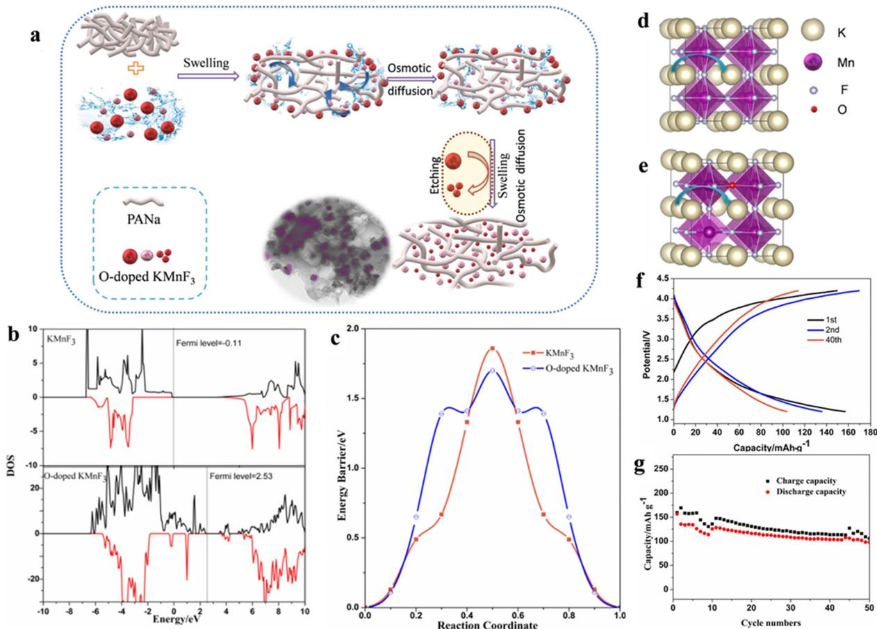
Fig. 9 Schematic diagram of the synthesis process. (a) Charge/discharge curves (b) and cycling performance (c) of  $\text{KMnO}_{0.125}\text{F}_{2.875}$ . Spin polarization of DOS (d) and energy profile (e). Schematic diagram of K migration (f and g).<sup>110</sup> Copyright © 2020 Elsevier.
