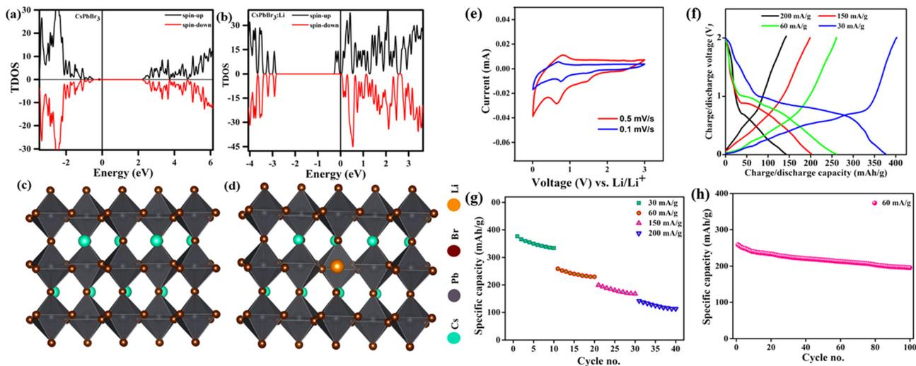
Fig. 2 TDOS of CsPbBr<sub>3</sub> without (a) and with Li<sup>+</sup> (b). Side views (c and d). CV curves (e), GCD curves (f), specific discharge capacity (g), and cycling diagram (h) of CsPbBr<sub>3</sub>.<sup>48</sup> Copyright © 2021 American Chemical Society.
