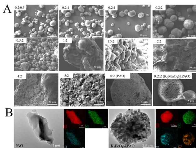
Fig. 2 SEM images of  $K_2FeO_4@PAO$  with different  $K_2FeO_4$  and PAO contents (A) and TEM image and EDS mappings of PAO and  $K_2FeO_4@PAO$  (B). The preparation conditions for  $K_2FeO_4@PAO$  are shown in Table 1.
