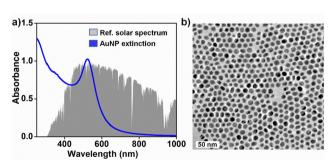
Fig. 1 (a) UV-visible absorption studies show a strong overlap between the surface plasmon band of AuNPs (centred at  $\sim$ 520 nm) and the solar spectrum, confirming the suitability of sunlight as the irradiation source. The solar spectrum was adapted from the ASTM G173-03 AM1.5G reference spectrum with permission. (b) A representative transmission electron microscope (TEM) image of 12.0  $\pm$  0.4 nm AuNPs.
