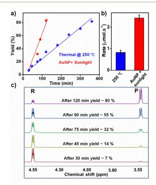
**Fig. 3** (a) A plot showing the variation in the product yield with respect to time for plasmonic-heat (red) and electrical-heat (blue) driven Claisen rearrangement. (b) The bar diagram showing the corresponding reaction rates. (c) A plot showing the variation in <sup>1</sup>H-NMR signal with respect to time for plasmonic-heat driven Claisen rearrangement (only the region covering the distinguishable peaks of reactant and product is shown for clarity).
