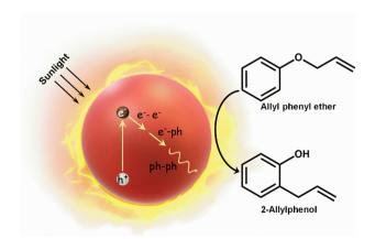
Scheme 1 Schematic representation of plasmonic-heat driven Claisen rearrangement of allyl phenyl ether to 2-allylphenol. The photoexcitation of plasmonic AuNPs leads to a series of nonradiative processes: Landau damping, electron-electron  $(e^--e^-)$ , electron-phonon  $(e^--ph)$ , and finally heating-up the local environment via the phonon-phonon (phph) interactions. This heat dissipated from the plasmonic AuNPs was used as the thermal energy source for the Claisen rearrangement.
